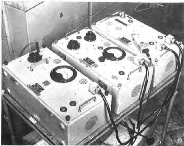
Left—Level measuring set. Centre—Oscillator. Right—Power unit FIG. 5—WIDEBAND TRANSMISSION MEASURING SET STC 74602
