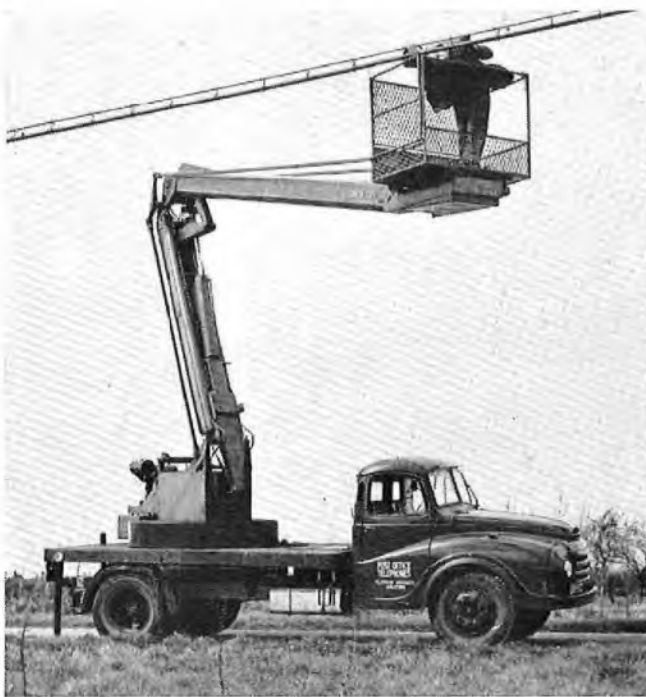
FIG. 5—HYDRAULIC ELEVATING PLATFORM IN USE
