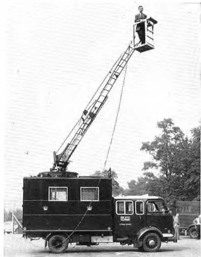
FIG. 3—LADDER ROTATED, ELEVATED AND EXTENDED
