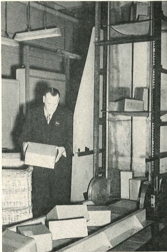
FIG. 4—EXPERIMENTAL MODEL OF THE POST OFFICE VERTICAL ELEVATOR
