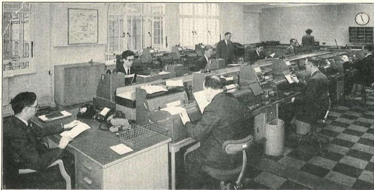
FIG. 5.—DISTRIBUTION DESK AND TELEPRINTER AUTOMATIC TRANSMITTING POSITIONS. SHELL-MEX HOUSE.
