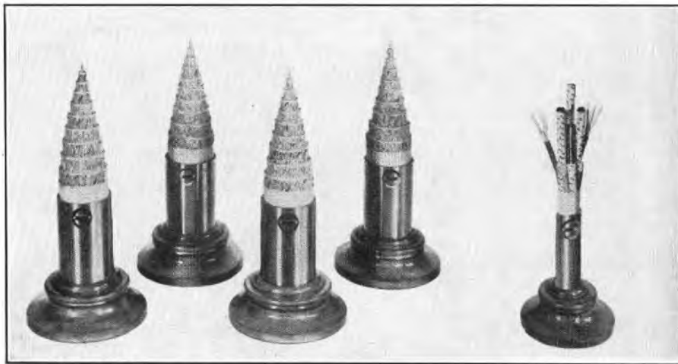
FIG. 7.—CABLE PROGRESS—COAXIAL CABLE ON THE RIGHT WILL PROVIDE MORE CIRCUITS THAN THE FOUR AUDIO-FREQUENCY CABLES ON THE LEFT.
