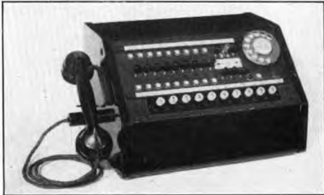
FIG. 20.—CORDLESS SWITCHBOARD USED WITH P.A.B.X. No. 1.
