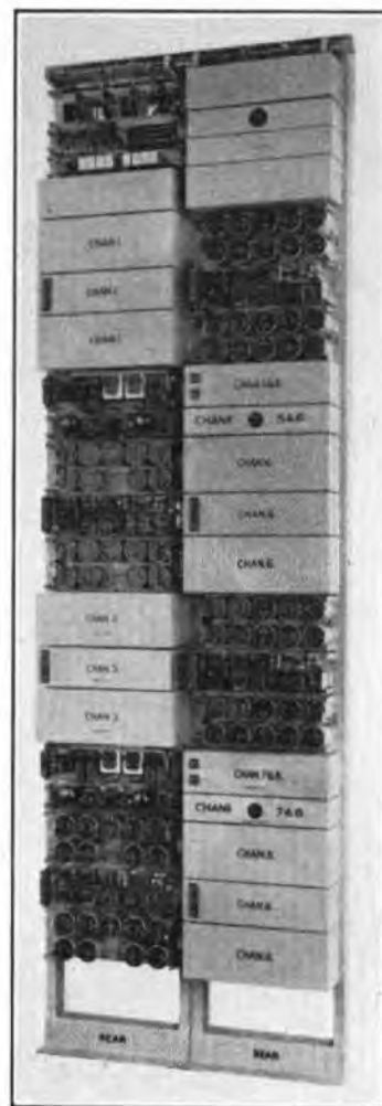
FIG. 5.—CARRIER SYSTEM NO. 5—CHANNEL EQUIPMENT.
