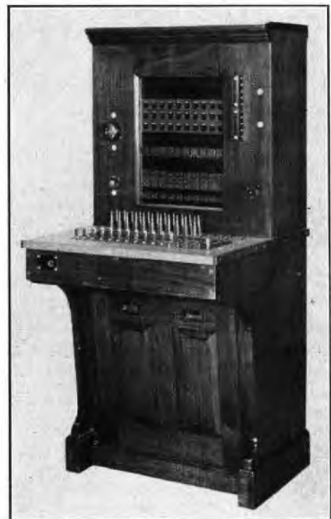
FIG. 16.—EARLY CORD SWITCHBOARD.
