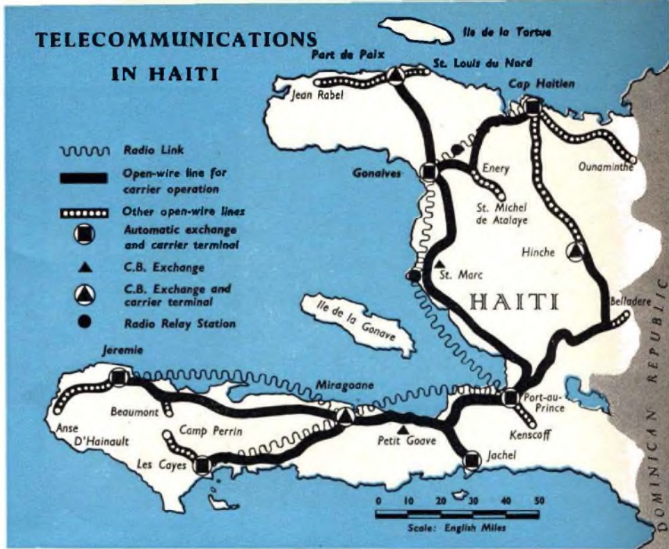
The network of open-wire lines, radio links and exchanges in Haiti. This system is one of the many systems throughout the world for which G.E.C. is responsible for the planning, manufacture and installation.
