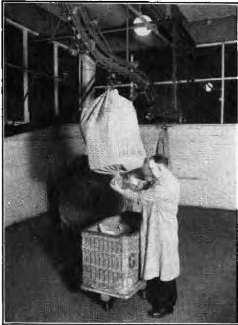
FIG. 4.—BAG OPENING FROM A CHAIN CONVEYOR.
