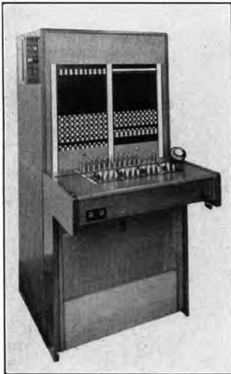
FIG. 18.—MODERN LAMP-SIGNALLING SWITCHBOARD (P.M.B.X. No. 1A).
