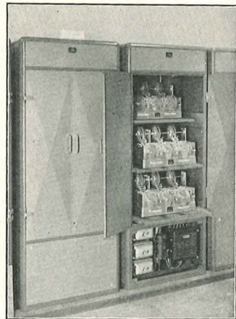
FIG. 2.—AUTOMATIC NUMBER TRANSMITTERS.
