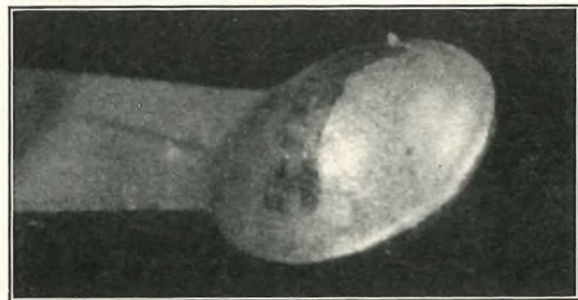
(a) Mechanical Wear on Wiper after 1,000,000 Calls
