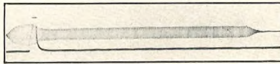
(d) Wiper with Unpolished Rhodium-Plated Tip.
