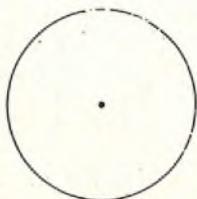
(b) POLAR DIAGRAM IN PLANE PERPENDICULAR TO LINE OF DIPOLE i.e., EQUATORIAL PLANE
