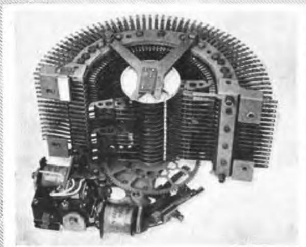
The High-Speed Motor Uniselector which operates at 200 outlets per second.
