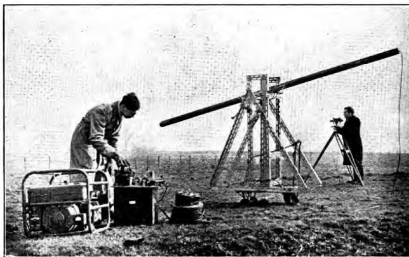
FIG. 4.—METHOD OF SUPPORTING MAGNET ASSEMBLY DURING CALIBRATION.
