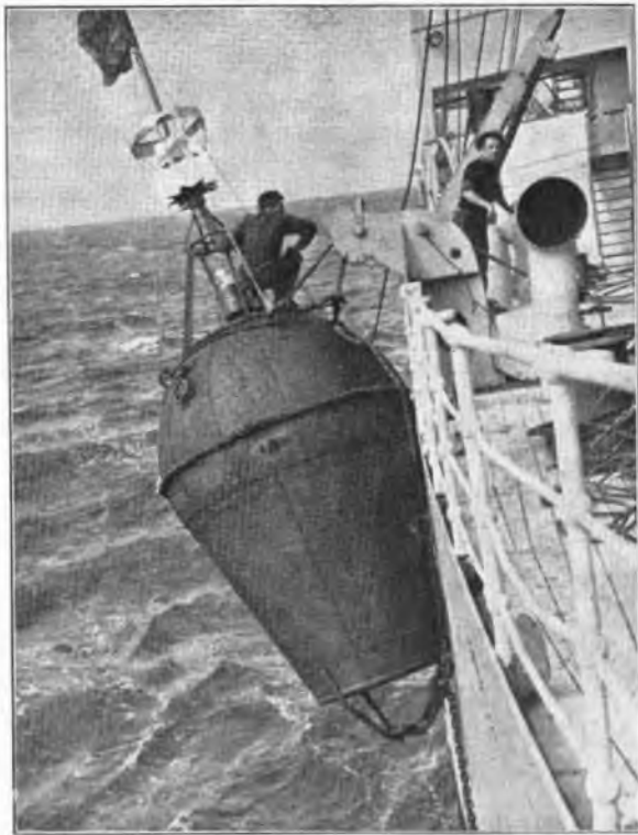
FIG. 5.—BUOY HOISTED TO DECK LEVEL ON SPECIAL SHEAVE.
