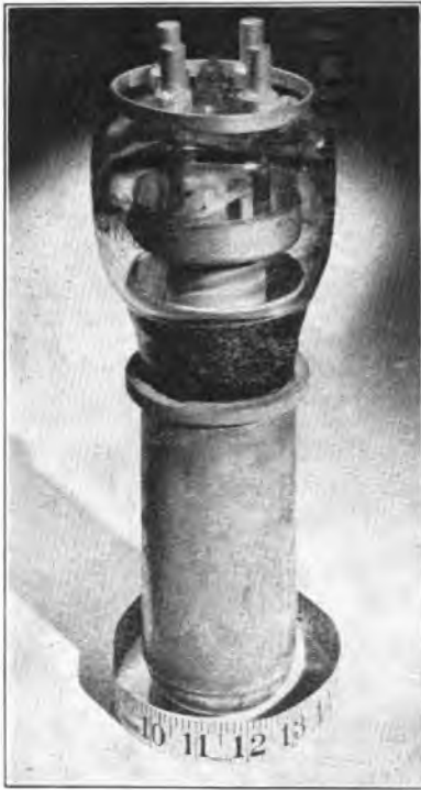
FIG. 3.—SINGLE-ENDED 20-KW WATER-COOLED TRIODE WITH THORIATED-TUNGSTEN FILAMENT.
