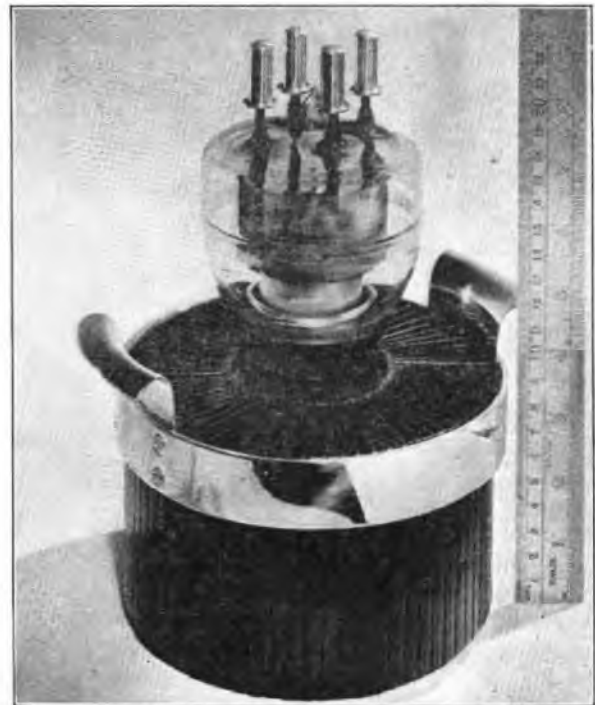
FIG. 6.—FORCED-AIR-COOLED TRIODE, 4.5 kW ANODE DISSIPATION.
