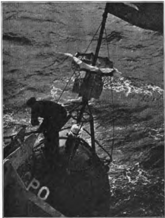
FIG. 4.—SEAMAN SHACKLING 6 X 3 ROPE FROM BOW SHEAVE BEFORE MOORINGS ARE SLIPPED FROM BUOY AT SIDE SHEAVE.
