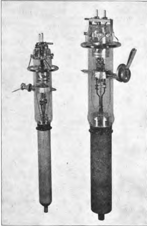
FIG. 5.—18-kW TRIODE (RIGHT) AND 12-kW TRIODE, WITH SIDE-ENTRY GRID SEALS.
