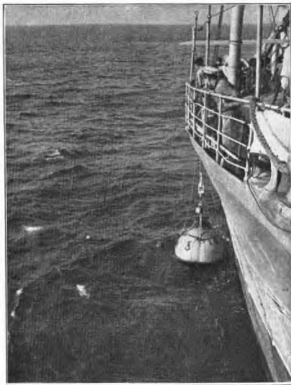
FIG. 3.—VIEW, LOOKING AFT, OF BUOY COMING IN ALONGSIDE SHIP AND SEAMEN HOOKING "TAIL" WITH GRAPNELS.
