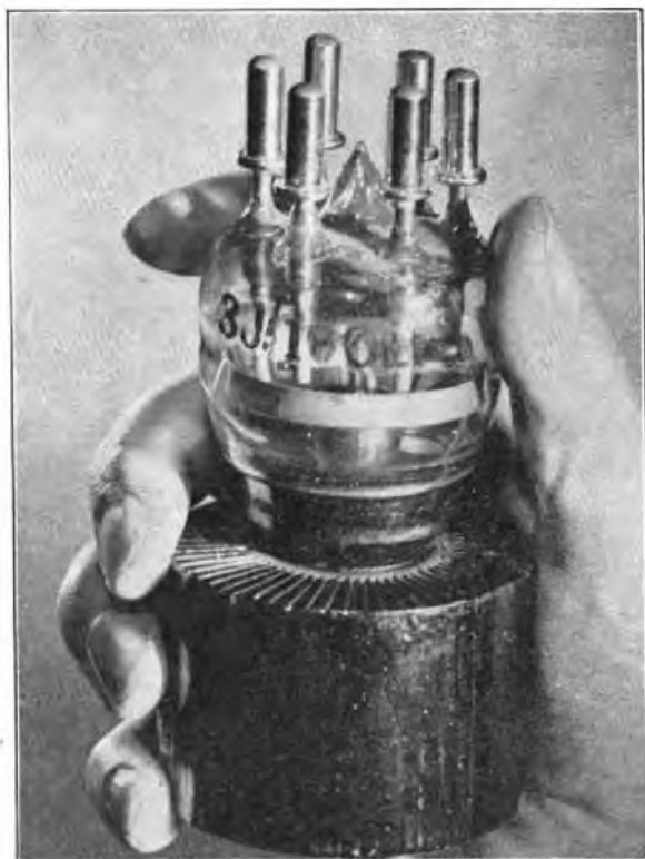
FIG. 7.—FORCED-AIR-COOLED TRIODE, 1 kW ANODE DISSIPATION.
