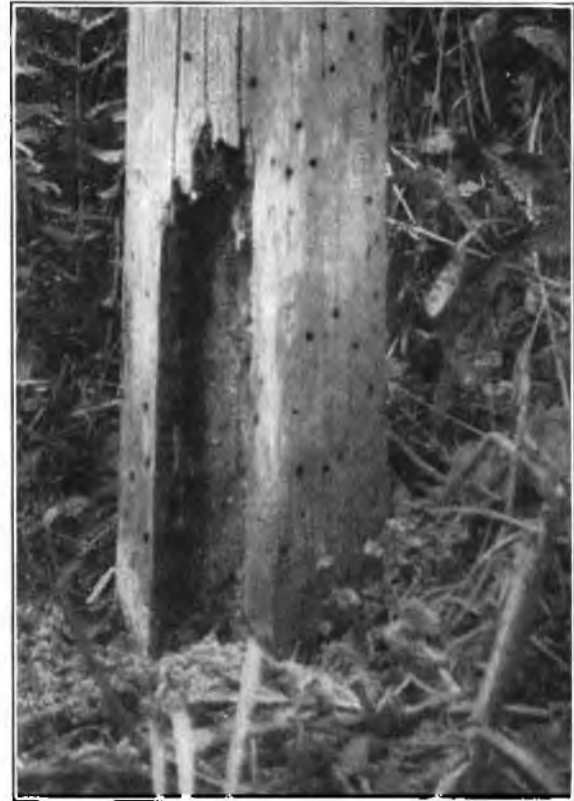
In a few short weeks, the larvæ of Rhagium can transform a pole classified as "S" into a potential accident trap for an unwary lineman.
