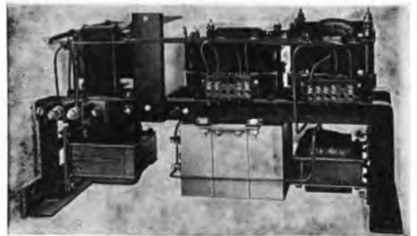
Type "B" Stabilistor with cover removed.
