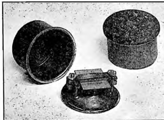
FIG. 2.—CRYSTAL PLATE MOUNTED IN EVACUATED METAL CONTAINER.
