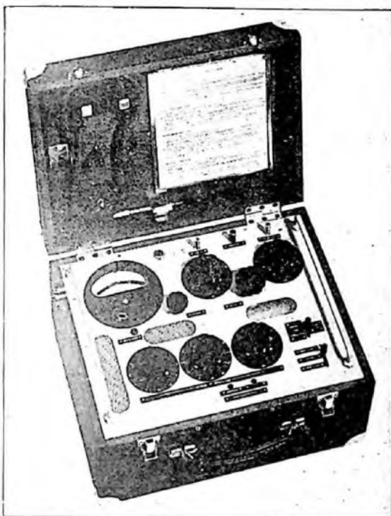
FIG. 1.—H.F. TRANSMISSION MEASURING SET.
