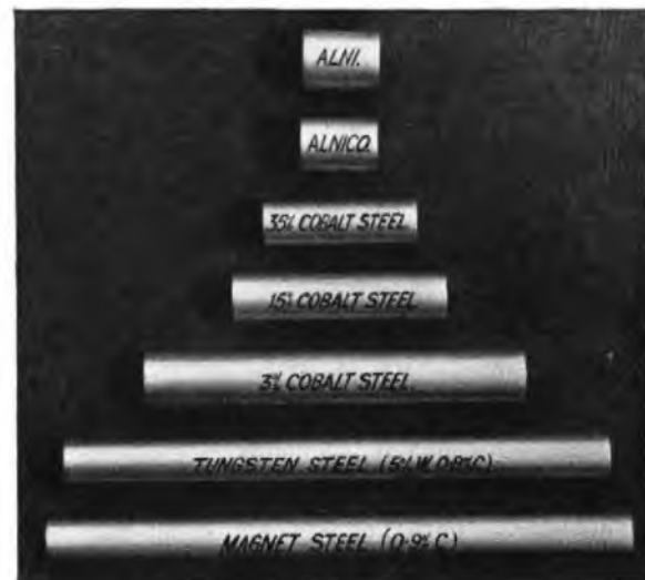
FIG. 5.—RELATIVE SIZES OF BAR MAGNETS IN VARIOUS ALLOYS TO PRODUCE A SPECIFIED FLUX DENSITY.
