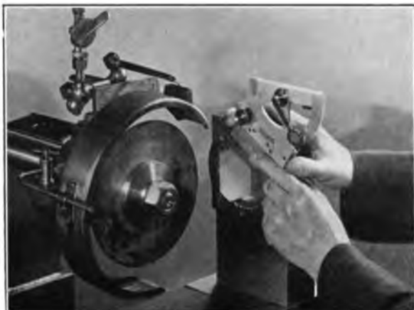
FIG. 18.—SETTING UP Z SLABS WITH CLINOMETER.
