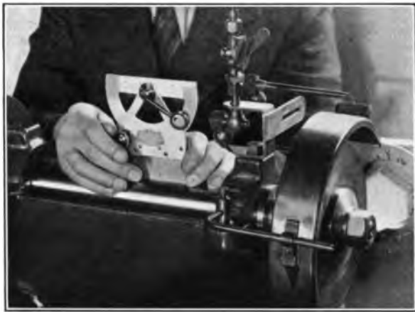
FIG. 17.—CHECKING MACHINE SPINDLE LEVEL WITH CLINOMETER.
