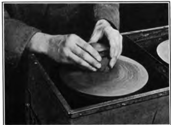
FIG. 24.—GRINDING SLAB ON ROTARY LAP.
