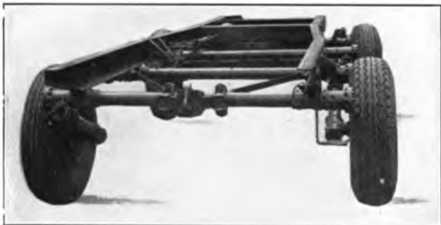
FIG. 3.—TORSION BAR TRAILER CHASSIS.
