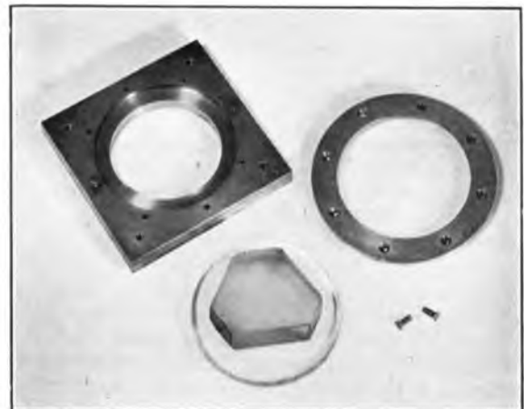
(b) FIXTURE PARTS AND Z SLAB MOUNTED ON GLASS DISC.
