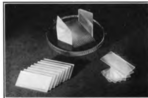
(b) X PLATES REMOVED FROM Z SLAB AND CLEANED.
