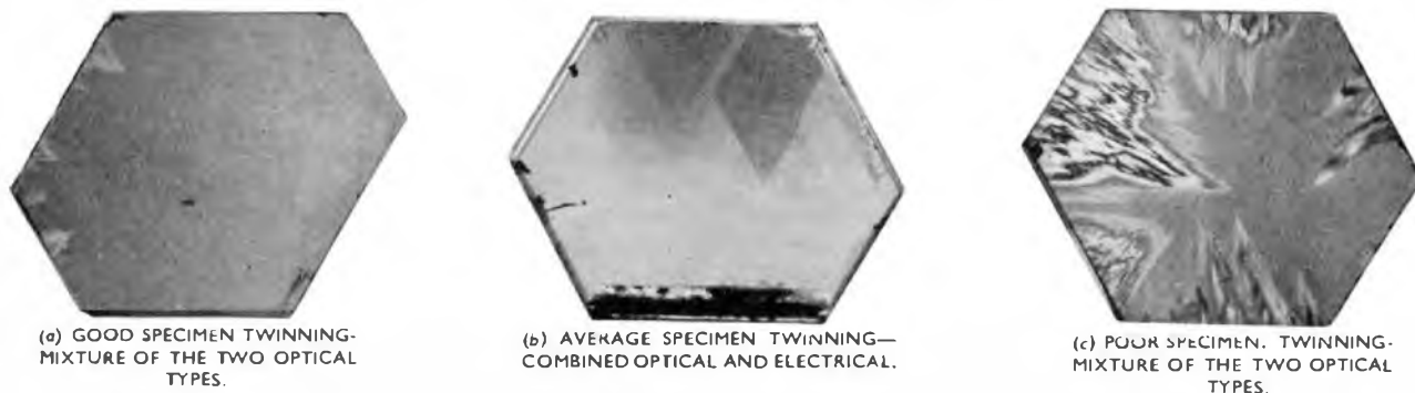
FIG. 11.—Z SLABS IN PLANE POLARISED PARALLEL LIGHT.
