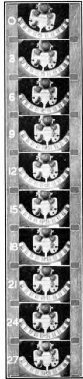
FIG. 8—EXTRACT FROM FILM SHOWING OSCILLATION OF AUTOMATIC SELECTOR WIPER.
