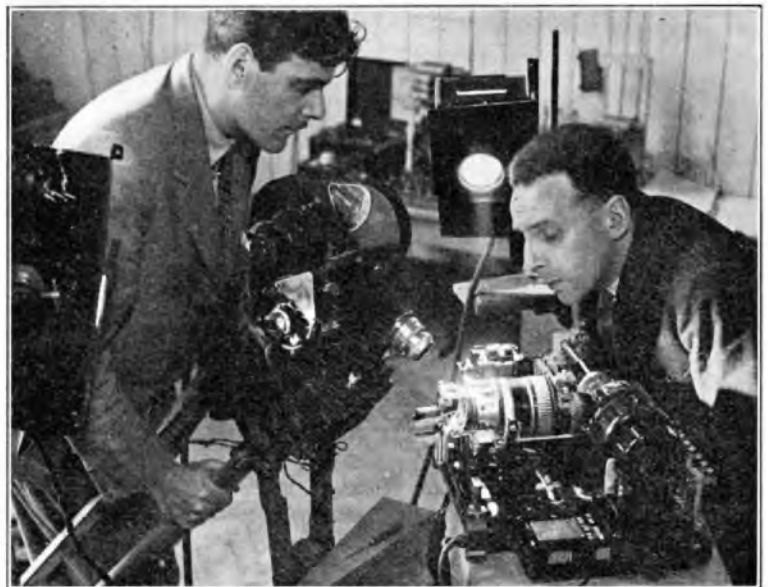
FIG. 6.—TAKING HIGH SPEED FILM OF A TELEPRINTER MECHANISM.
