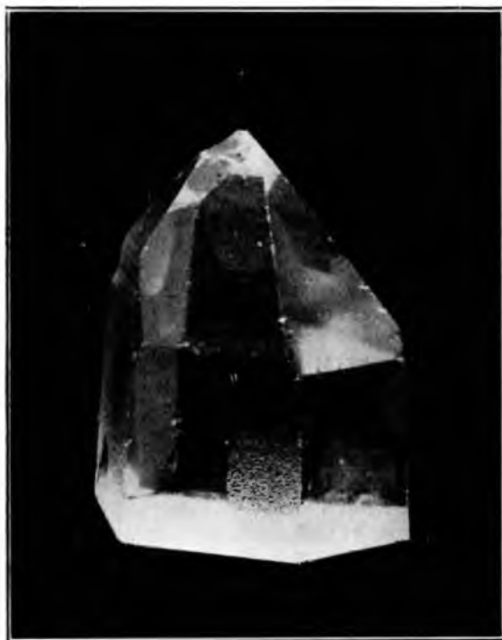
(a) NATURAL ETCH PATTERNS ON PRISM AND PYRAMID FACES.
