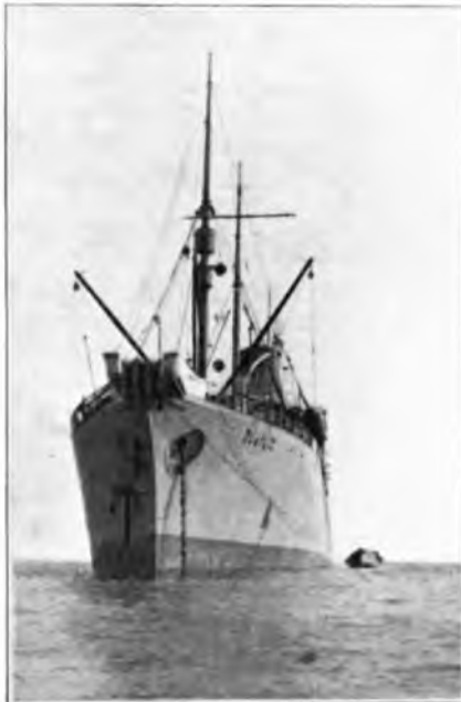
FIG. 3.—THE "DOMINIA'S" BOW SHEAVES.
