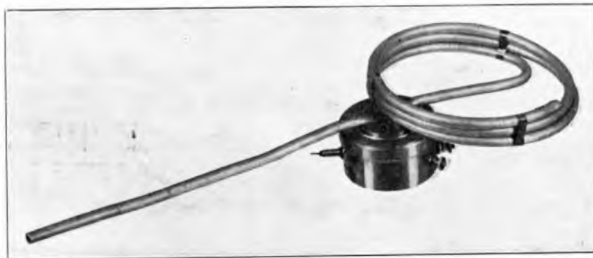
MOUTHPIECE ATTACHMENT TO CONDENSER TRANSMITTER FOR MEASURING SOUND PRESSURES AT A POINT.
