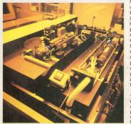
The production of the glass master at Sonopress. The information from the tape, via a laser beam, is written on the glass master. MUSIC & MEDIA - May 23, 1987
