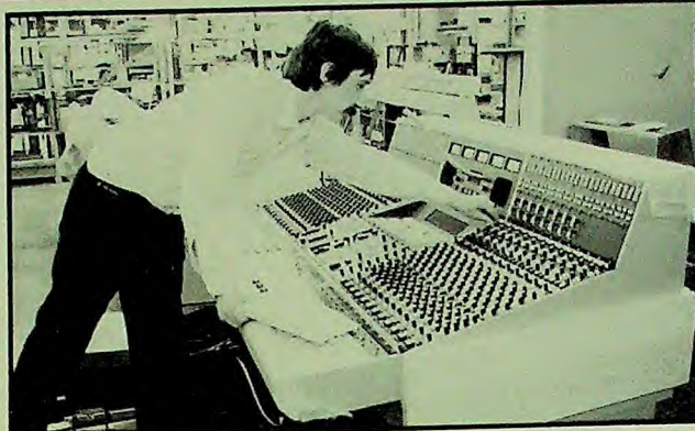
A NEVE console in the making, at the factory in Melbourn, Cambs.
