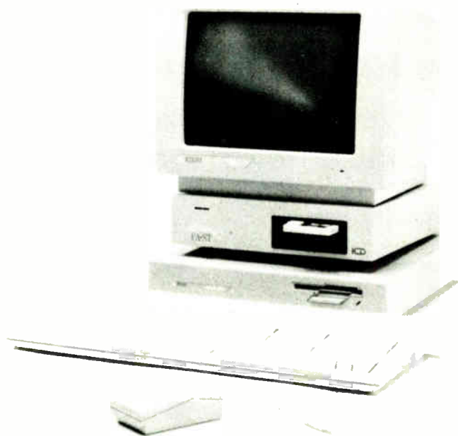
ICD's FA-ST tape backup allows you to back up data from your ST's hard disk onto high density data cassettes.
