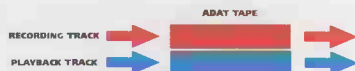
The ADAT format records each track discretely, as all professional multitrack recorders should.
