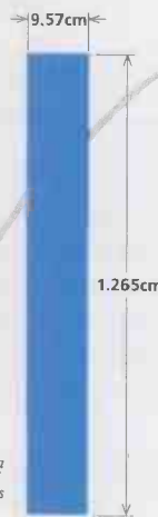
The total tape area for every second of ADAT operation is 1,211mm 2 .
