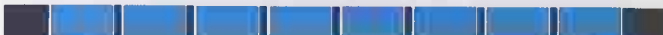
An ADAT's helical scan: ADAT tracks are safely separated into 8 discrete data blocks.
