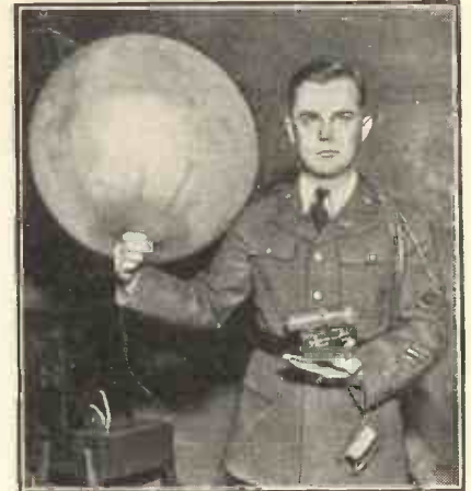
Weighing only one pound, this U.S. Army transmitter is carried by a hydrogen-filled balloon and automatically transmits meteorological data to observers on the ground.
