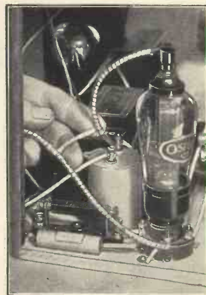
The metal shielding on all the screened leads has to be earthed. In the case of the anode lead to the S.G. valve, this can be effected by twisting the end of the metal ribbon round the adjacent screened lead.
