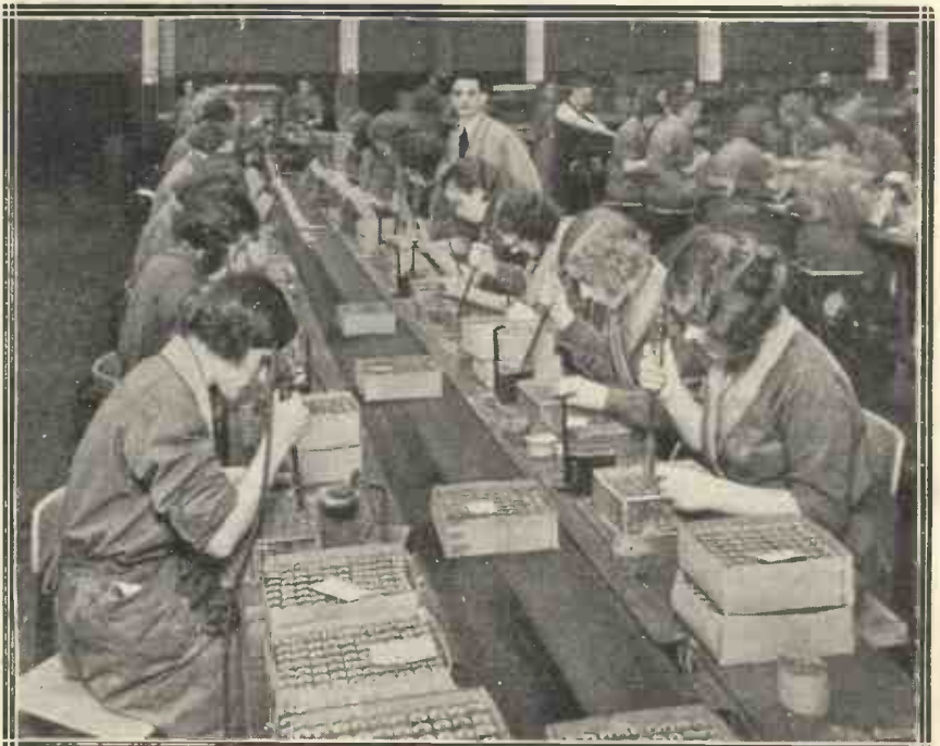
Part of the army of girls at work in the new Ever Ready factory at Walthamstow. They are busily engaged in connecting up the groups of cells in H.T. batteries. Note the belt conveyor system running down the centre of the bench.
