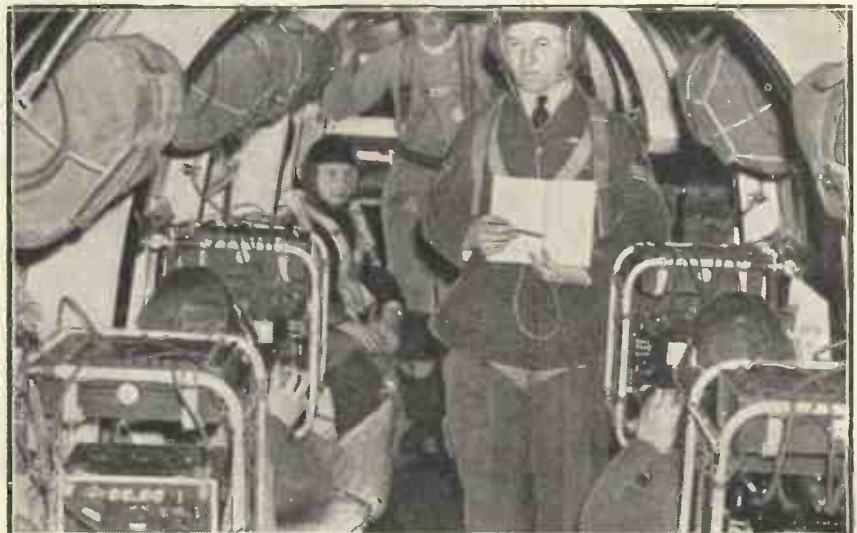
So that they will have practical experience of aeroplane wireless, R.A.F. students of radio technique receive part of their instruction in a Vickers Victoria machine equipped to carry an instructor, five pupils, and the necessary sets of apparatus.
