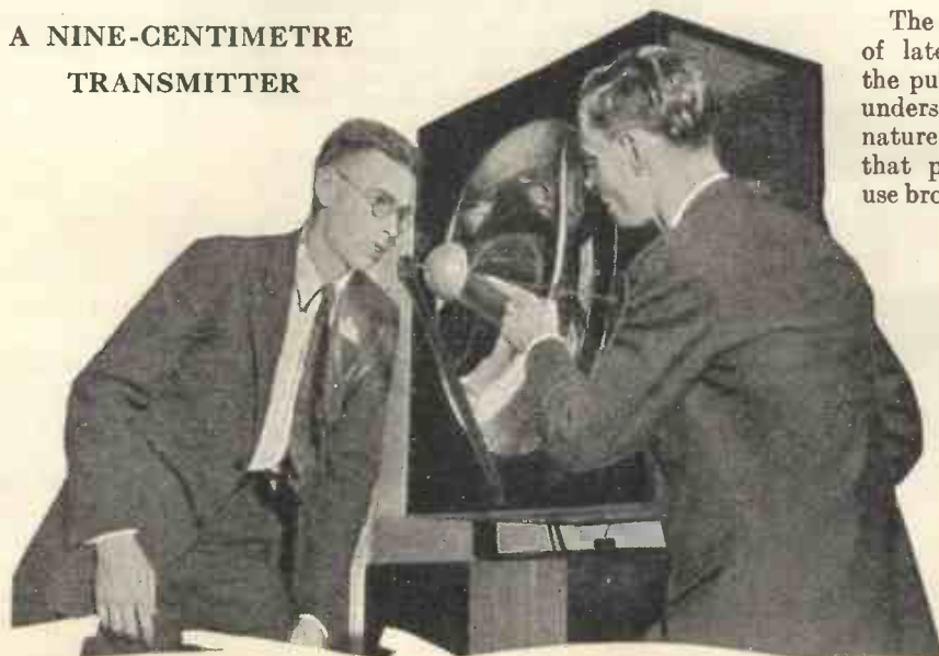
This radio apparatus, shown at the Century of Progress Exposition in Chicago, has been aptly christened the "Beamcaster." The waves employed are only nine centimetres long and are projected by the parabolic reflector behind the short aerial to which the engineer is pointing.
