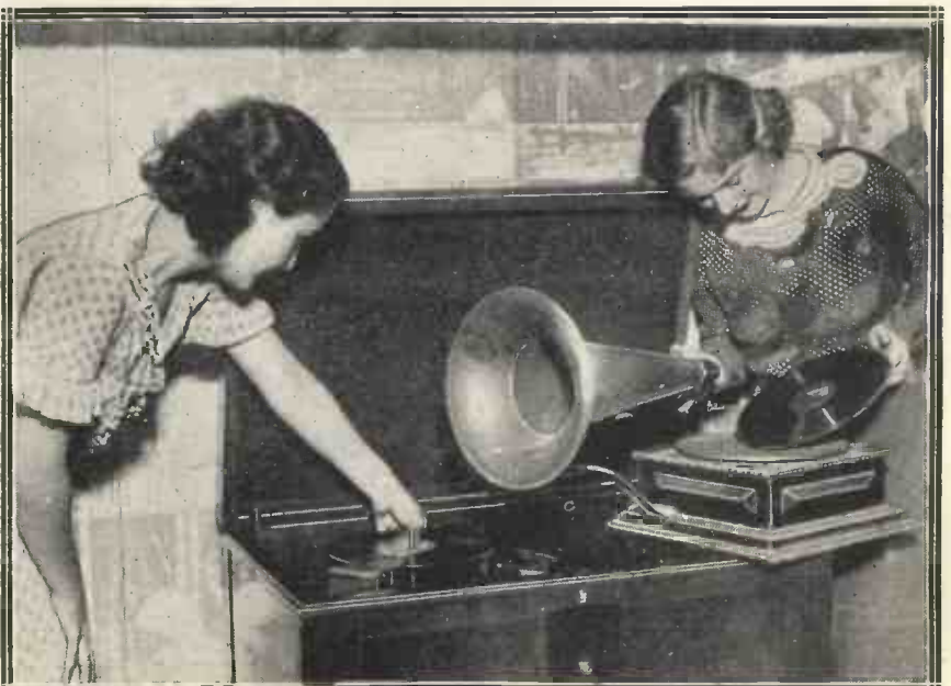
Here is an interesting comparison—a horn type gramophone of thirty-five years ago and the latest H.M.V. radio-gramophone, which plays up to eight records continuously.
