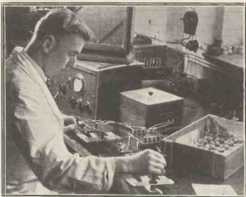
"Iron dust" coils of the Ferrocart type always undergo stringent matching tests. The engineer seen above is checking up the various coils with an oscillator unit and loud-speaker. The final inductance adjustment is made by altering the distance between the two halves of the coil.
