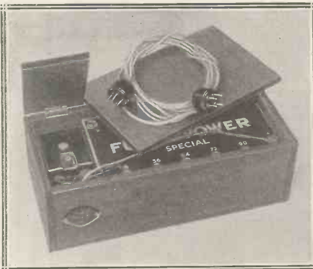
The top of the battery box, apart from the hinged portion that gives easy access to the accumulator, is normally screwed into place. Twin armoured cabling is used for connections between the battery box and the set.
