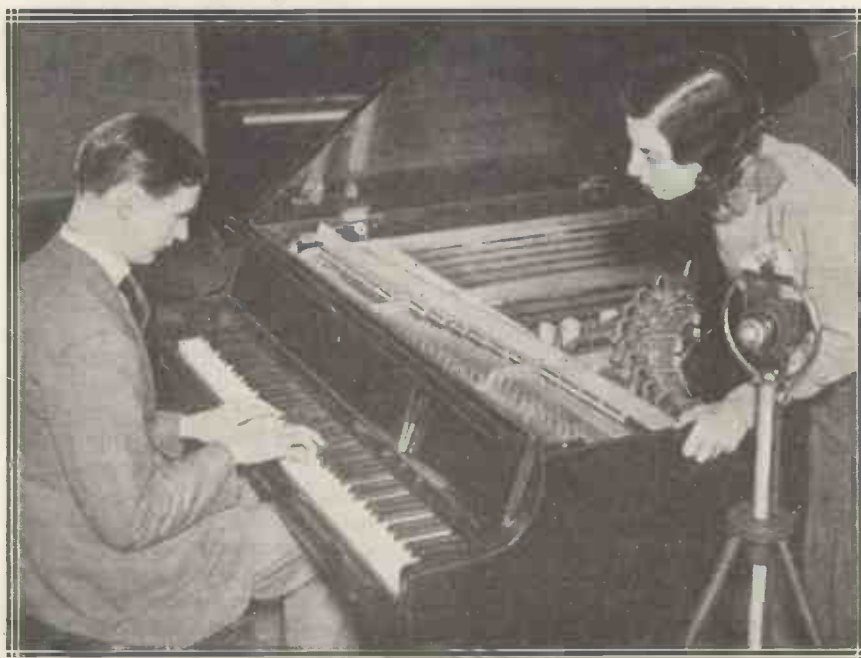
THE NEO-BECHSTEIN piano is an instrument in which the reproduction has a similarity to that of an organ. The sounds from the strings are picked up by microphones, passed through an amplifier and then applied to a loudspeaker. Here we see John Hunt recording a Chopin prelude at the H.M.V. studios.
