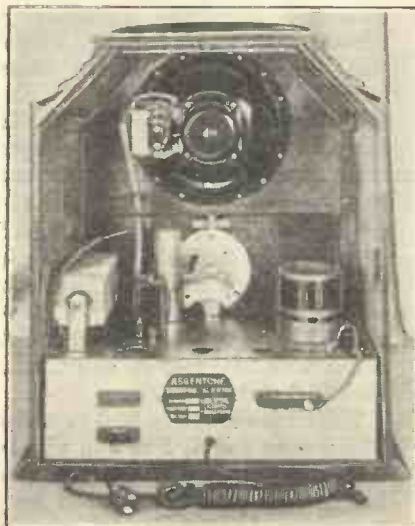
The mains rectifier for high-tension can be spotted to the left of the chassis, while to the right is the inductance.
