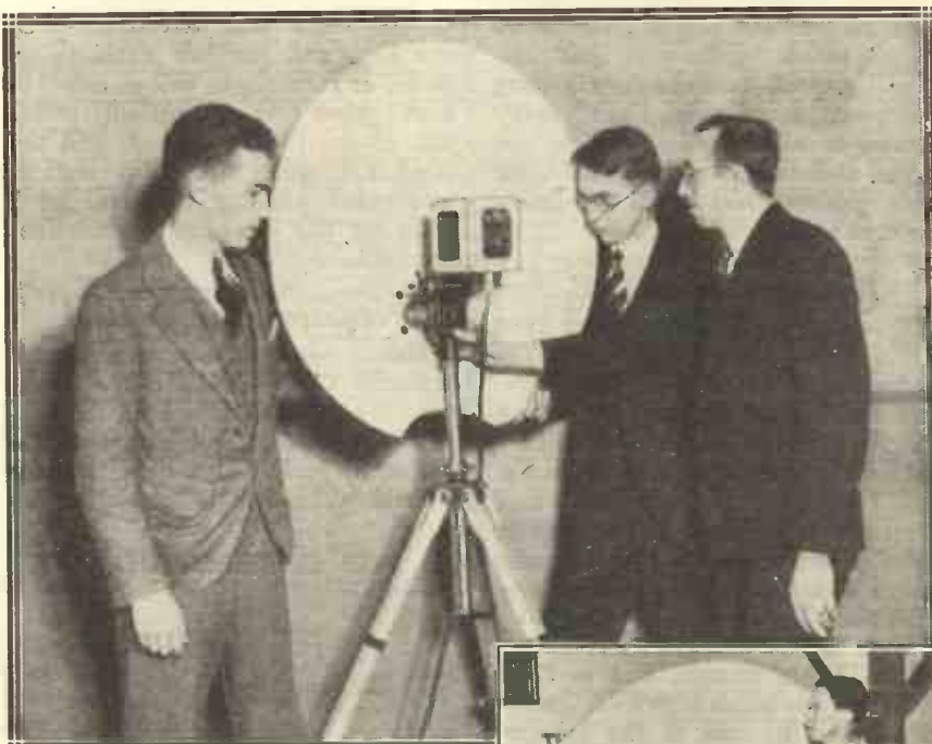
Although looking rather like some micro-ray apparatus, the instrument in the top photo is actually a microphone assembly for use in large halls, the reflector being used to concentrate sound in the microphone. Below are seen the two sizes of reflectors which have been used very successfully.
