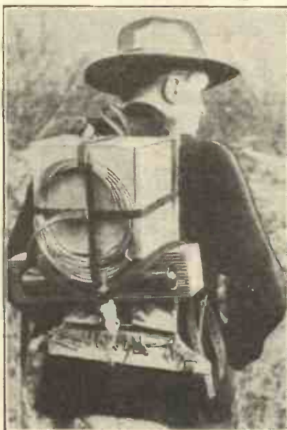
Part of the equipment of this forest "fire-lookout" is a complete portable transmitter and receiver, which is used for reporting and communication during fires.
