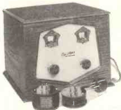
A short-wave adaptor made by Messrs. Hustler, Simpson & Webb. (Stand 30.)
