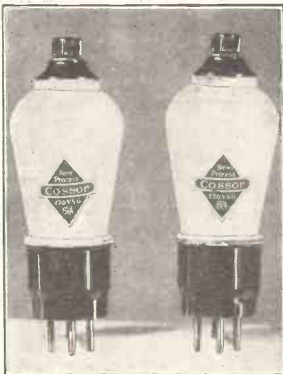
Two of the first of the British variable-mu valves. They are Cossor battery types. (Stand 60.)
