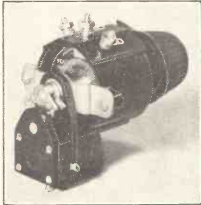
A combined volume control and on-off switch by Wearite. (Stand 82.)
