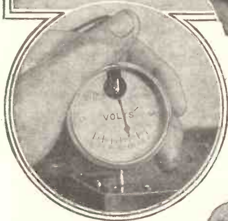
(In Circle.) Use a high-resistance voltmeter to test H.T. batteries, and take special care to do your testing with the set switched on.
