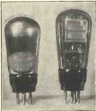
Here are two little giants in the pentode class—the Marconi P.T.2 and the Mazda 220Pen.
