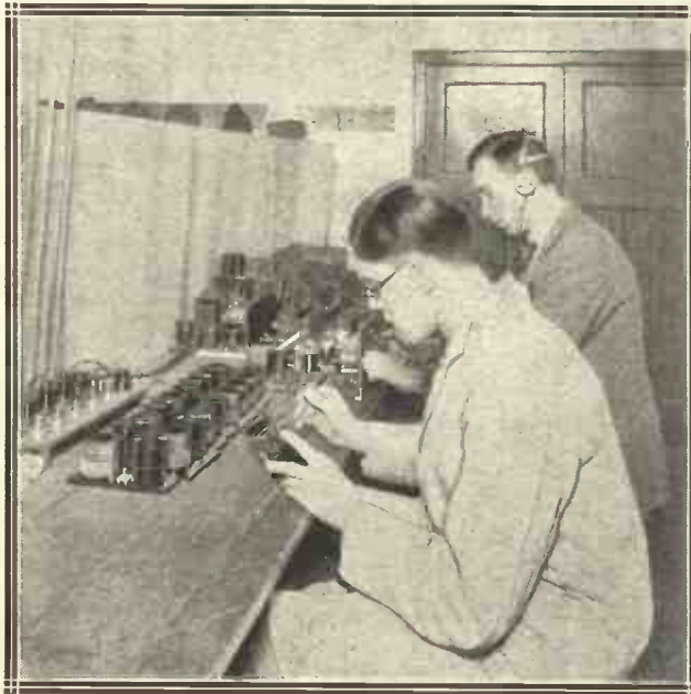
Although home-wound coils sometimes give trouble, there is little possibility of faults occurring after rigid testing like this. Not only do these commercial coils each receive careful inspection and measurement, but they are also tested on actual signals in a set.
