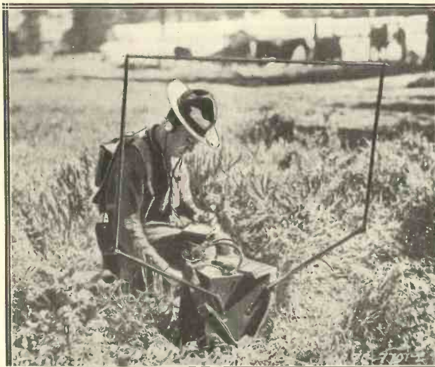
The American Army authorities are very keen on portable radio equipment, and here you see one of the special field short-wavers in operation. Note the handy loop-aerial, which can be easily folded for transport purposes.
