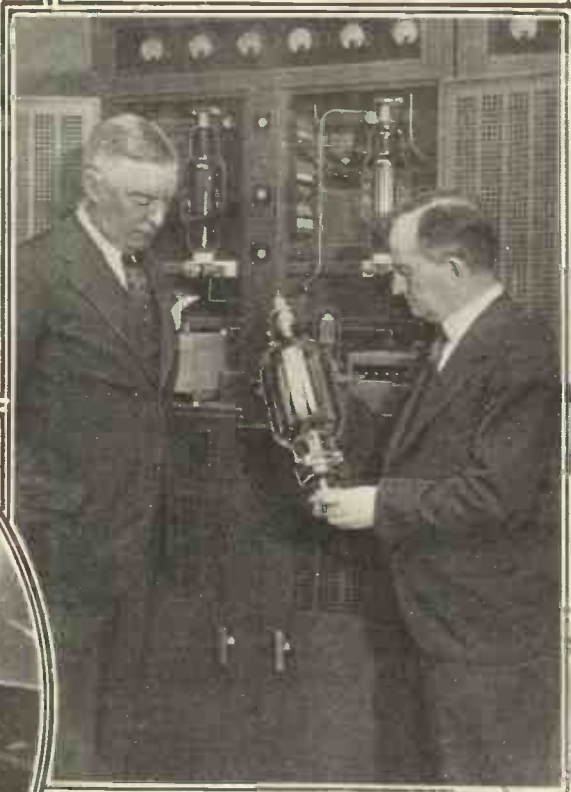
The picture above shows one of the valves at Police Headquarters, removed from the transmitter for inspection.
