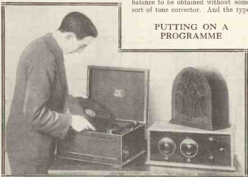
This photograph shows the "Eckersley" Three being used with the H.M.V. Playing Desk No. 116 and the L.S.7 moving-coil speaker.
