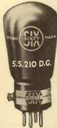
Here are the T.C.C. 2-mfd. condenser, a Six-Sixty double-grid valve, and a Coszor metallised S.G. valve.
