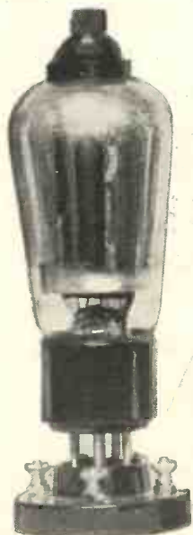
This mains S.G. valve has a magnification factor of 1,500—a colossal figure.
