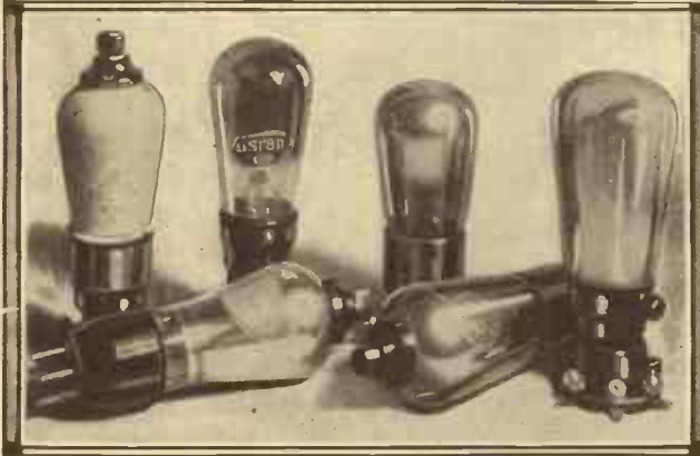
A group of well-known two-volt valves, including Coszor S.G., Osram H.2, Six-Sixty and Eta L.F. valves, and Mazda pentode.
