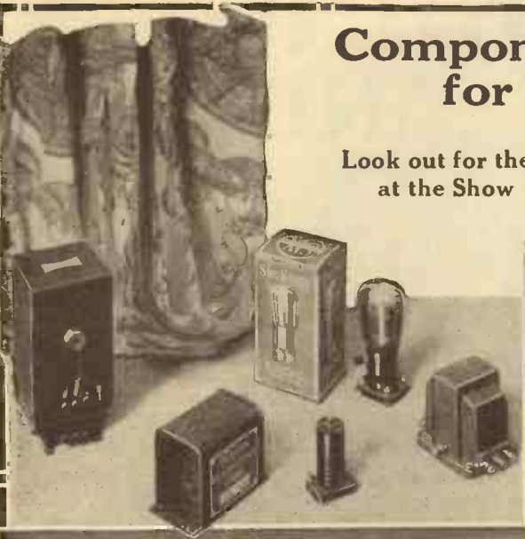
An interesting group comprising the Heyberd trickle-charger, Bulgin filter choke, Six-Sixty pentode valve, Lewcos H.F. choke, and Telsen output transformer.
