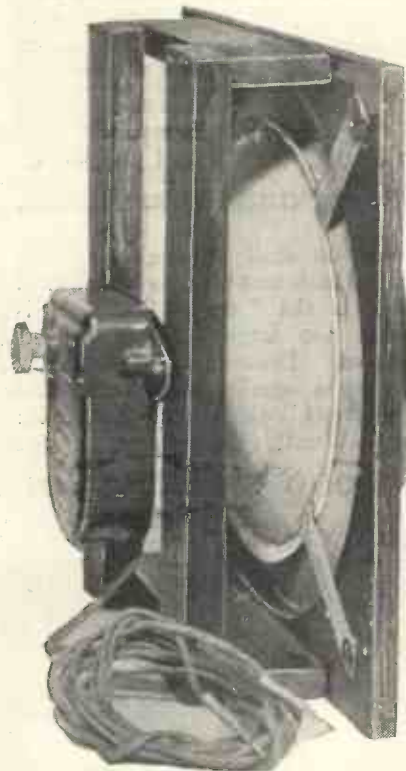
Most speakers of the type using an ordinary armature unit, and known as cone speakers, require less power for a given volume than moving-coil speakers. The one illustrated here is the "Modern Wireless" "Inter-Axial" Junior, as described in the February issue.
