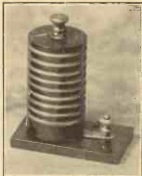
The Parex H.F. choke is popular and inexpensive.
