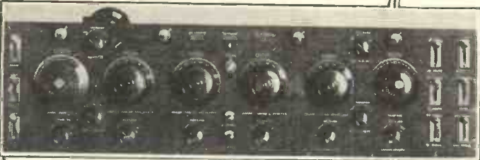
These two photographs show the control panel and the back of the receiver. The first dial from the left is the short-wave tuner, the next four belong to the medium and long wave-lengths, and the one on the extreme right is the reaction control. The short-wave coils can be seen at the far end of the bottom photo.
