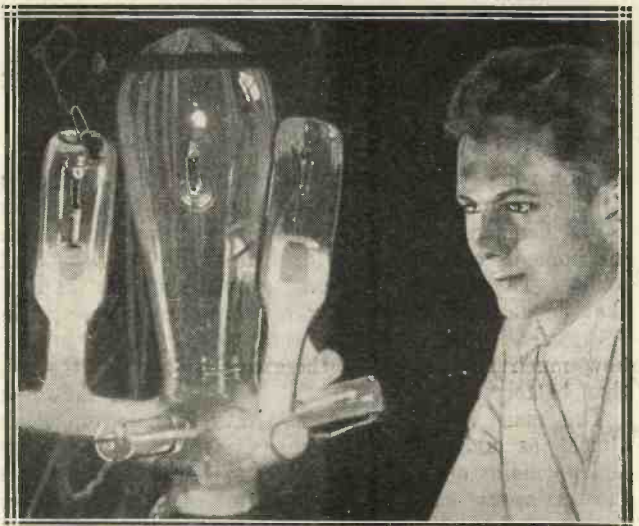
A new transmitting valve developed in America which can handle 30 amperes at 7,500 volts, and that is 225 kw. ! It is to be installed at K D K A, the famous short-wave broadcasting station.
