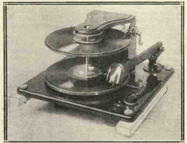
The Capehart record-changer undergoing tests at Tallis House. At the end of each record the pick-up lifts and comes out clear for the next disc to drop down.
