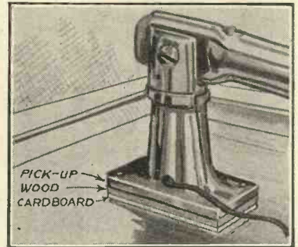
Having glued the wood block in position the pick-up is fixed to it with short screws. This makes a really firm and neat-looking job
