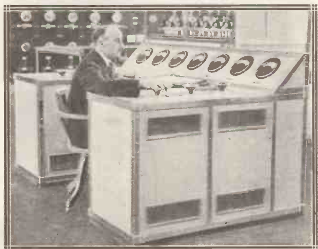
The control desk of one of the transmitters at Moorside Edge. From this position the engineer-in-charge has complete control of the whole transmitter, the row of meters in front telling him exactly what is happening in the various circuits.
