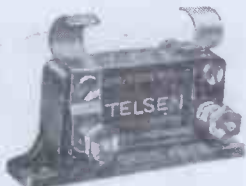
TELSEN FIXED (MICA) CONDENSERS , shrouded in Genuine Bakelite, made in capacities up to .002 mfd. Pro. Pat. No. 20287/30. .0003 supplied complete with Patent Grid Leak Clips to facilitate series or parallel connection. Can be mounted upright or flat. Tested on 500 volts. Price 1/- each.
