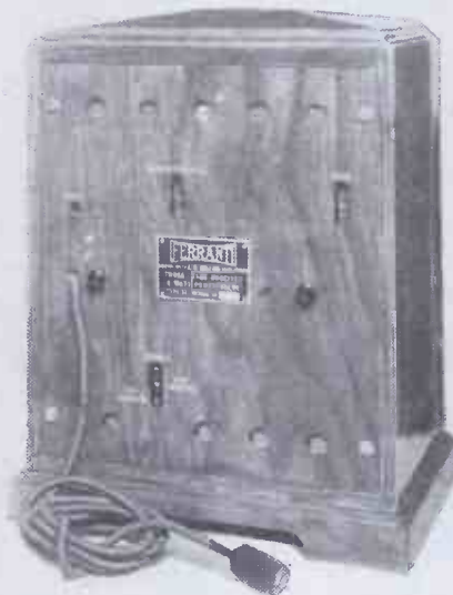
The back view of the Ferranti Three. Note the holes for ventilation and cooling of the A.C. valves.
