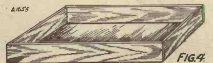
FIG. 4 The tray will prevent accumulator acid getting on to floors or carpets.
