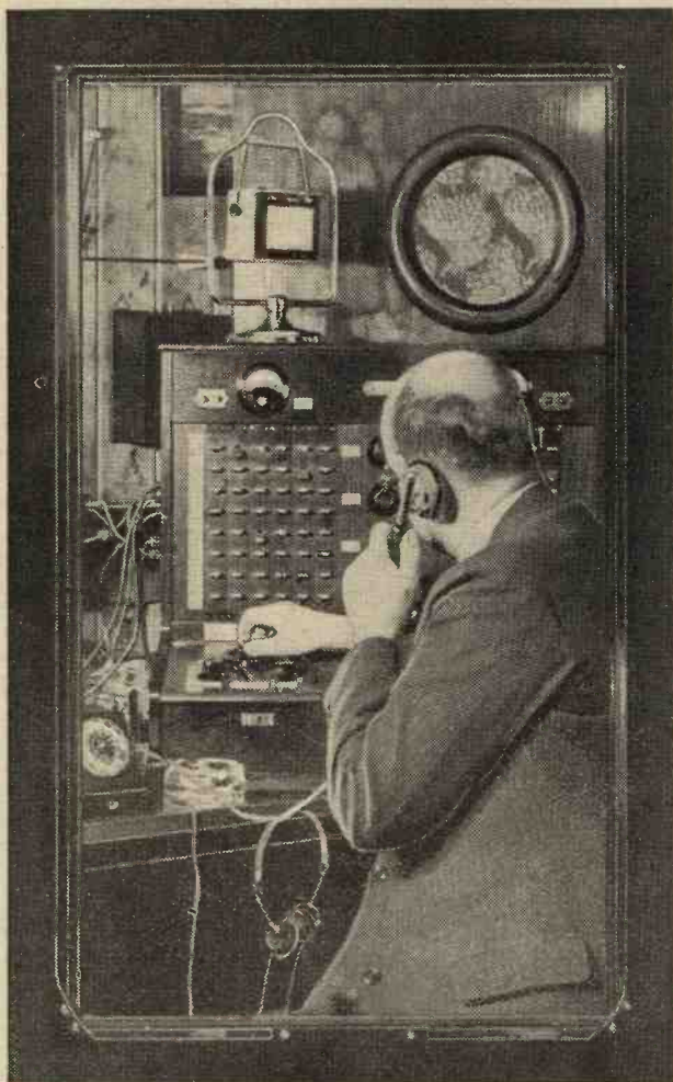
The chief engineer of the German State Broadcasting Corporation carrying out tests at his private house at Zehlendorf. All the German broadcasters can be connected by landline to this residence and various relay links arranged.
