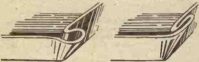
FIG. 1. FIG. 2. A1654 Showing how the lead is doubled in at the corners of the tray.
