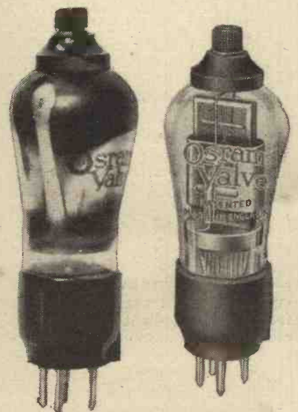
The battery and A.C. models of the Osram S.G. valve.
