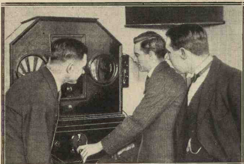
Receiving an experimental television transmission on one of the Baird combined sight and sound receivers. The received image appears at the back of the right-hand aperture and the left-hand one contains the loud speaker.
