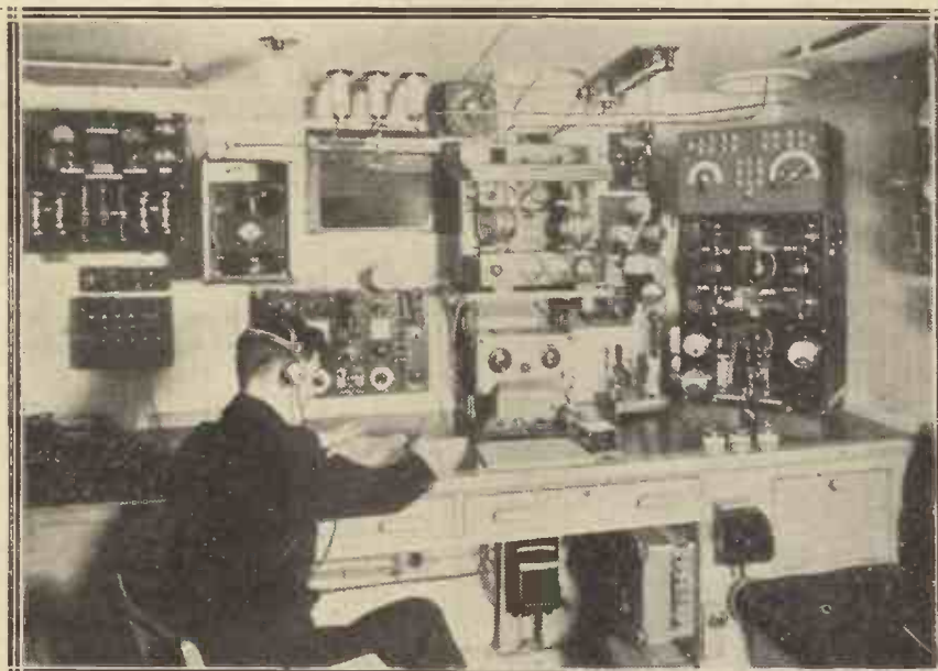
Special Marconi wireless equipment is installed on the new Royal Research Ship. Above is a view in the chart room which contains the direction finder.
