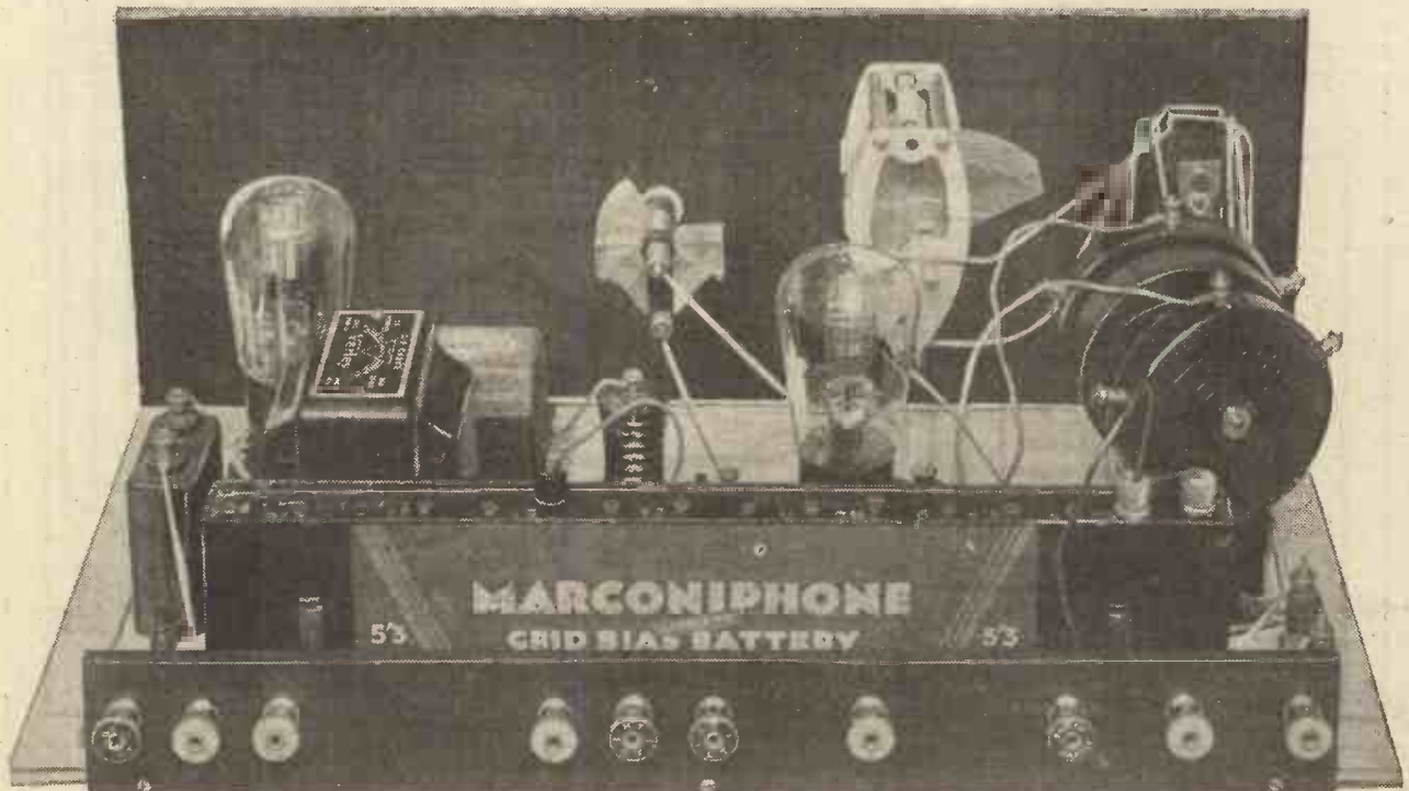
The only battery required for this set is the G.B. unit, which is fitted upon the baseboard. Note particularly the placing of the three coils.
