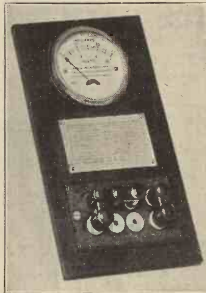
A universal meter, such as the one illustrated, will give you a sure indication of the state of your batteries, enabling you to take the voltage and also to check the bias points of the valves by watching the kicking of the milliammeter needle.
