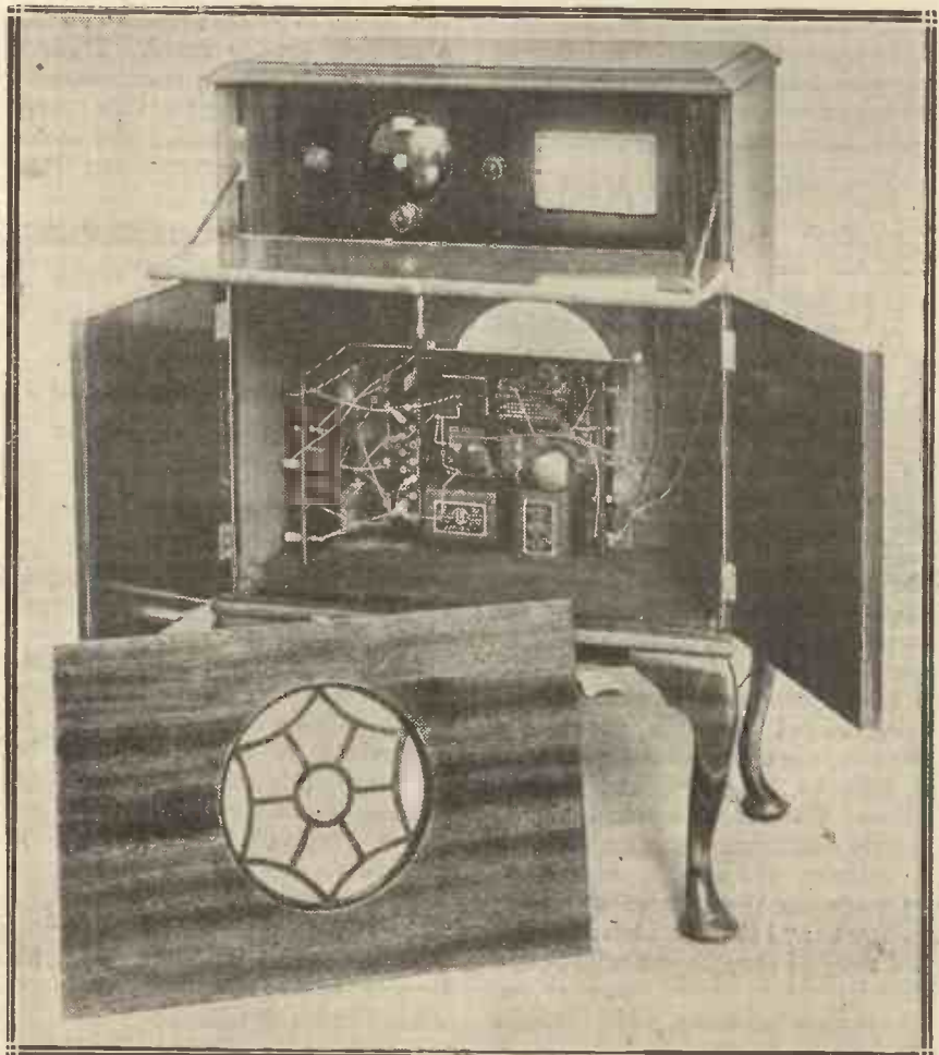
One method of assembling the set to form a handsome all-enclosed outfit is suggested here. The cabinet is one of Messrs. Pickett's standard lines, and the lower compartment houses the standard "M.W." A.C. power unit. Note how the latter is placed on its side to make room for a chassis-type loud speaker to be mounted on the detachable baffle board.
