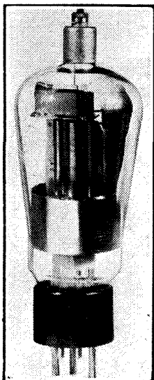
This Cosmos A.C. screened-grid valve is probably the most powerful H.F. valve yet placed on the market in any country. It has an impedance of about 800,000 ohms and a magnification factor of 1,200. It takes 1 amp. at 4 volts and gives tremendous magnification.
