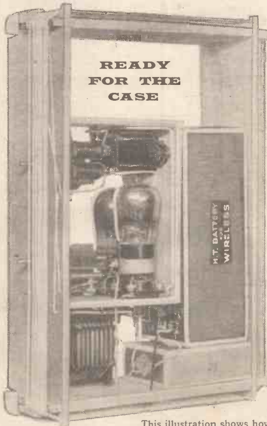
This illustration shows how the batteries are housed and the relative positions of the components. The frame aerial is wound round the wooden frame.
