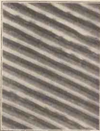
This photomicrograph shows a section of a gramophone record magnified 250 times, the indentations in the sides of the needle track representing the sound waves recorded thereon.
