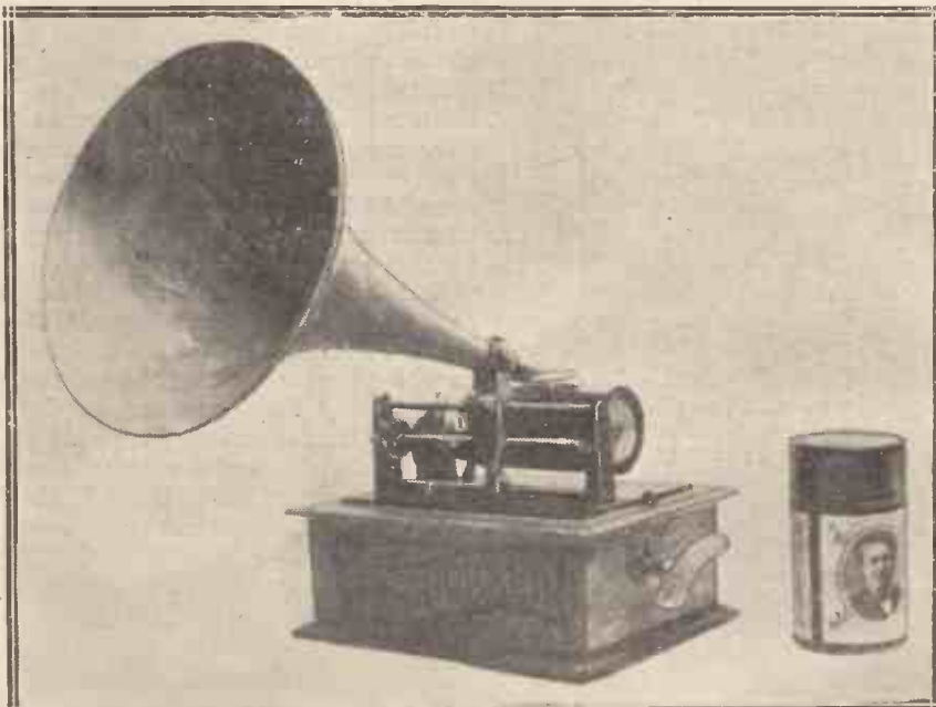
One of the very first phonographs, invented by Edison, and marketed in 1902. The records were cylindrical and were of fairly soft wax.
