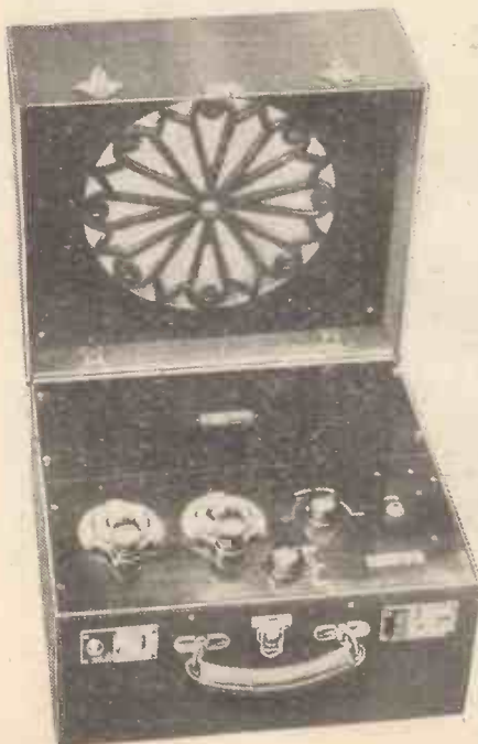
The "Lotus" portable uses an S.G. valve and has a fine range of reception.
