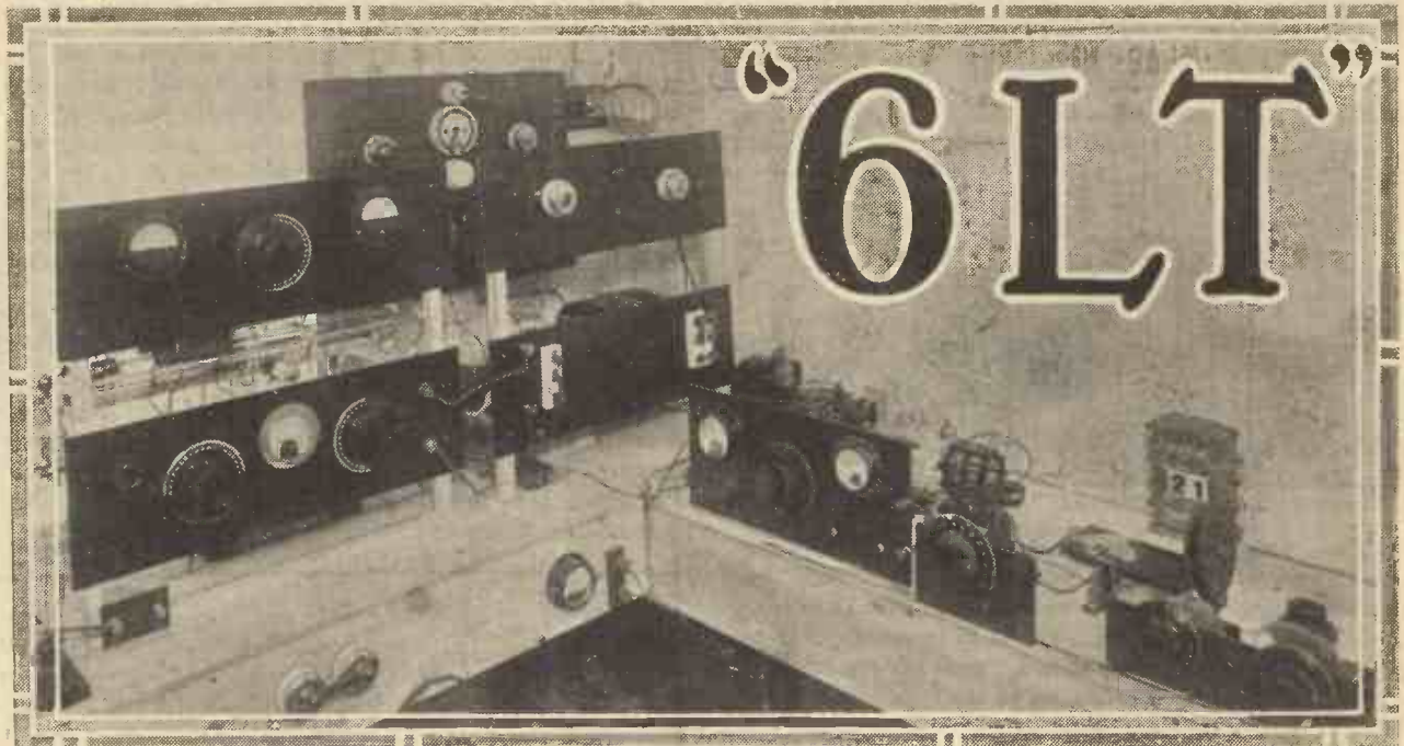
Details of a "baby" short-wave transmitter which is being used for tests where a portable station is essential.
