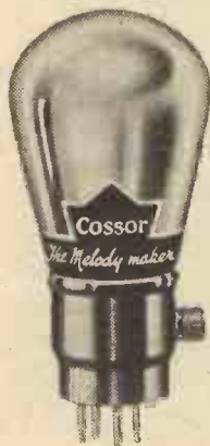
The Cossor Pentode valve. Note the terminal on the base, this terminal being for the connection to the priming grid.
