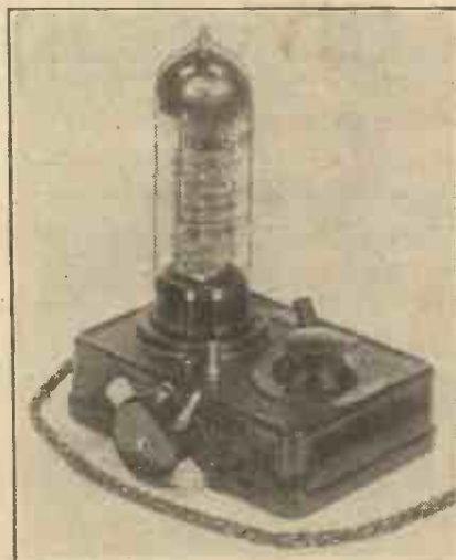
This is the Loewe triple-valve set, a feature of which is its extraordinary small size in comparison with the results given.
