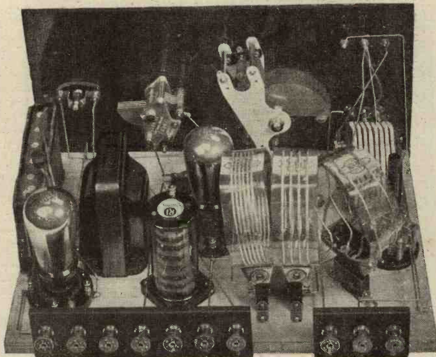
Here the set is shown removed from its cabinet, and with short-wave coils in position. In view of its versatility and efficiency its compactness and simplicity are somewhat staggering.
