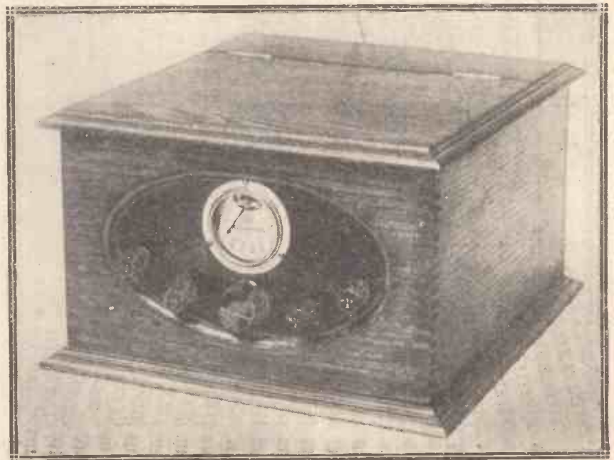
The milliammeter is connected in the last valve's plate circuit, where it helps to show the user any distortion due to overloading.
