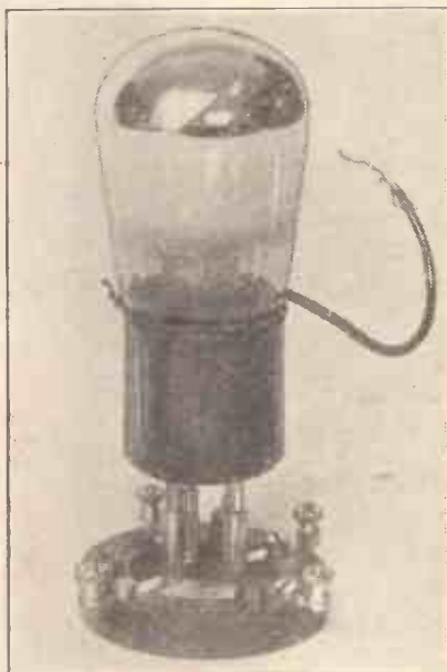
The Interdyne valve has a multi-electrode arrangement specially designed to provide a self-neutralising effect.
