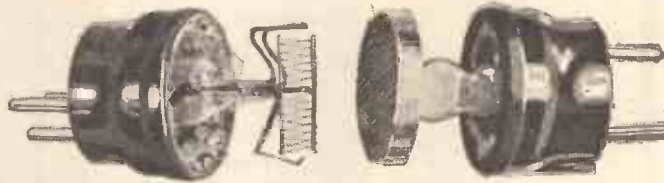
The assembly of one form of the screened-grid valve—a tetrode of amazing capabilities.
