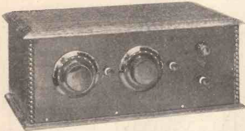
Beside each tuning dial is a wave-change switch, whilst to the right is the on-off switch, and above it the reaction condenser.
