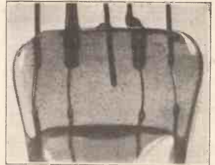
Fig. 4. The sealed "pinch" of a thermionic valve. (The centre support is for the unconnected end of the grid.)
