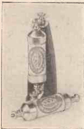
One of the new Lissen anode resistances, shown in a holder, together with a view of another in which the end terminals are clearly visible.
