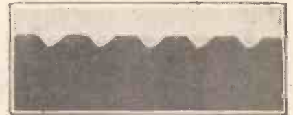
Magnified cross-section of commercial record showing the "U" cut. Some manufacturers prefer the "V" cut and some the "U" cut.
