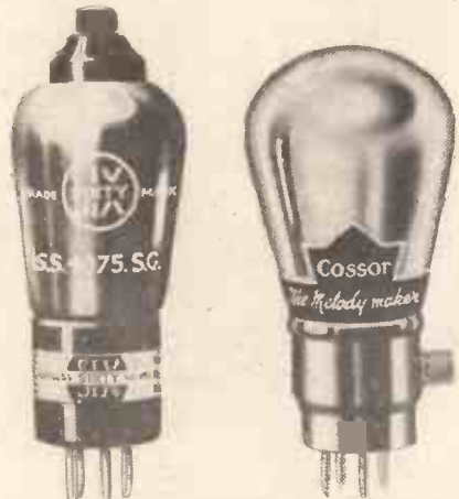
On the left is the Six-Sixty screened-grid 4-volt valve, and on the right the Cossor Pentode L.F. high-magnification amplifier.
