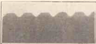
Magnified cross-section of a commercial record showing what is known as the "V" shaped cut. Notice that the width of the cut is approximately equal to the distance separating one groove from the next.
