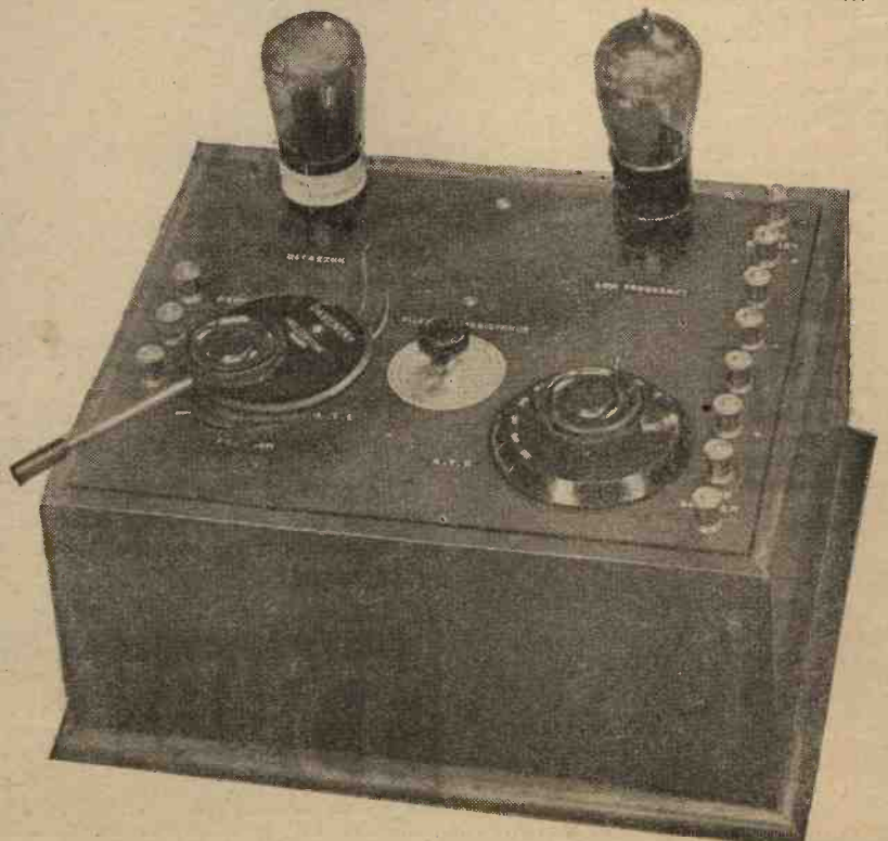
The "Sparrow" Two ready for test. A Daventry tuning unit is shown in position on the left of the panel
