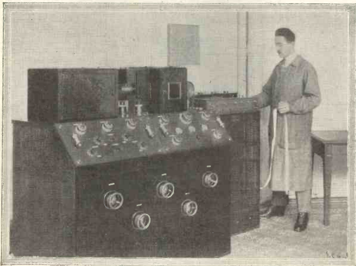
The recording of wireless signals at high speeds is one of the problems of long-distance commercial wireless work. This photograph shows the photographic recording apparatus in use at a great French wireless station.
