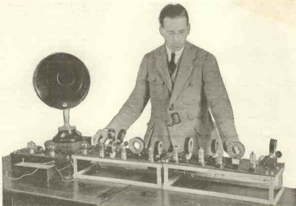
The author experimenting with a ten-valve receiver with seven stages of high-frequency amplification.
