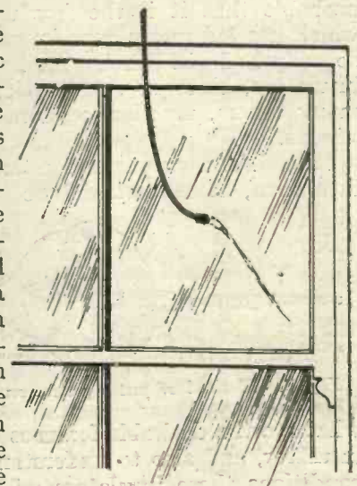
Fig. 4.—Using window pane as leading-in insulator.
