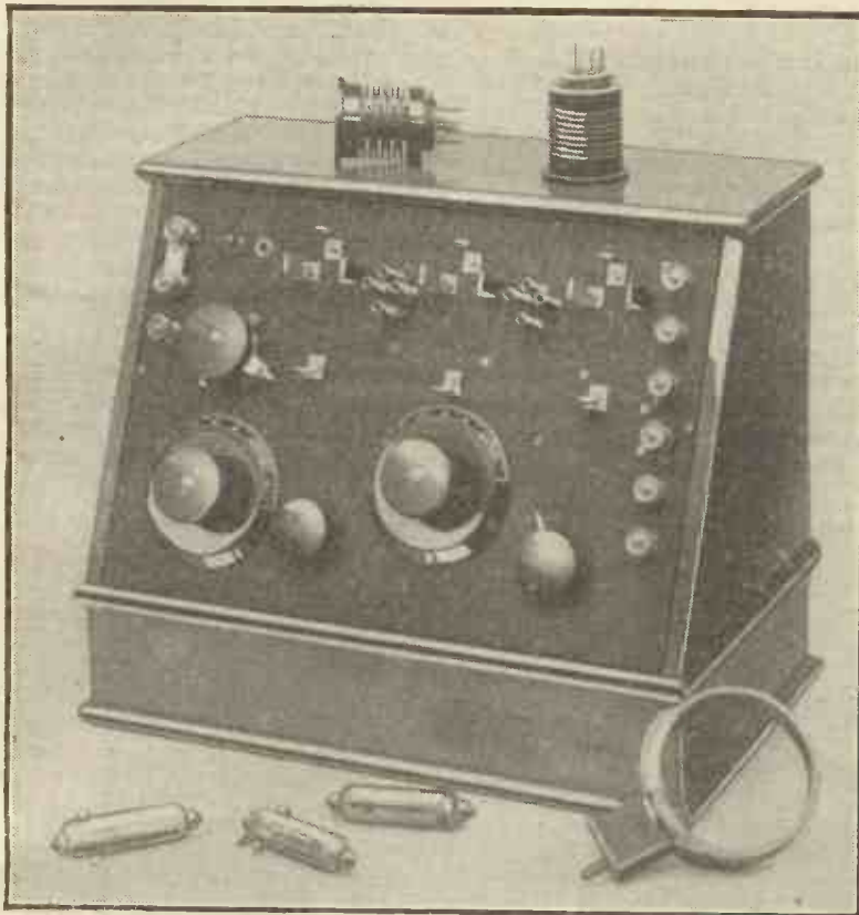
The set with valves, coil transformers removed to show construction.
