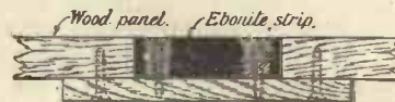
How to make joints in wireless cabinets. The bottom picture shows how to fit ebonite strips for terminals.
