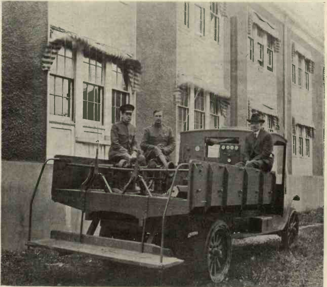
The above photograph was taken during some experiments with a Resonance Wave Coil Antenna carried out by the U.S.A. Signal Corps. Satisfactory telephony was carried out while the car was moving at 25 miles per hour.
