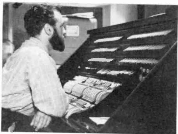
As the court action in The Verdict Is Yours switches from one part of the studio set to another, the studio lighting supervisor adjusts the lights from this keyboard which controls lighting.
