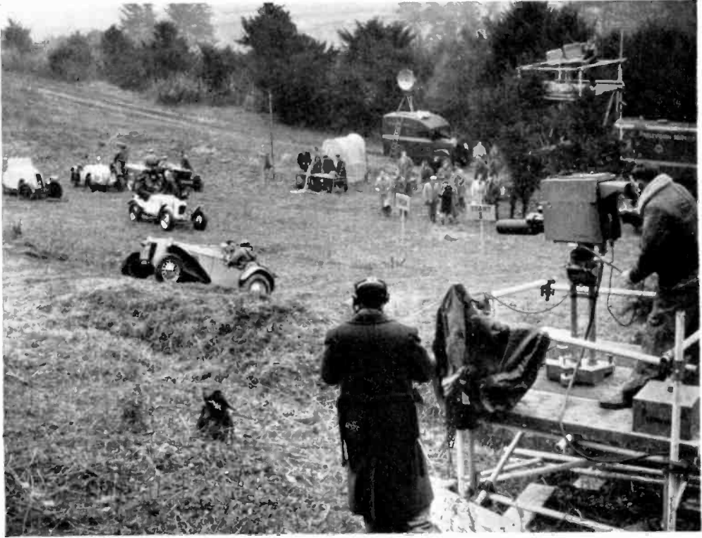
Television's outside-broadcast cameras are deployed to cover a motor reliability trial held in the Chiltern Hills. The set-up includes two cameras mounted on specially constructed platforms; the micro-wave transmitter, seen on top of the van in the background; commentator's tent, and mobile control-room.
