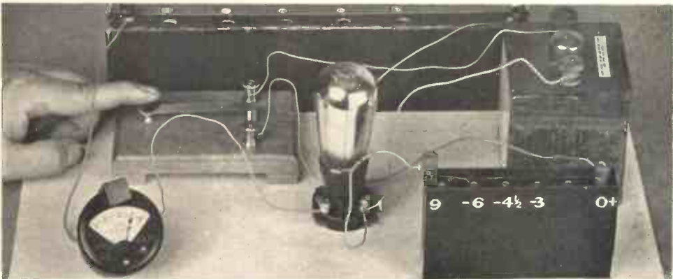
Fig. 26.—How THE ANODE CURRENT OF A POWER VALVE IS AFFECTED BY VARYING THE GRID BIAS This shows +9 volts applied to the grid, resulting in an anode current of 30 m.a.
