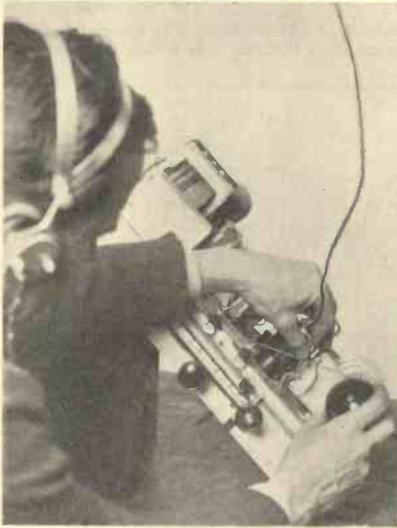
Fig. 1.—CONNECTING THE AERIAL TO GRID CIRCUIT OF DETECTOR VALVE TO ELIMINATE H.F. CIRCUIT.
