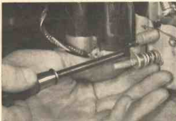
Fig. 8.—TAKING OUT THE PARKER-KALON SCREW WHICH HOLDS THE DIAL-DRIVE ASSEMBLY ON THE CONDENSER CASING.
