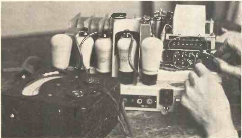
Fig. 20.—CHECKING UP THE MAINS TRANSFORMER WINDINGS.
