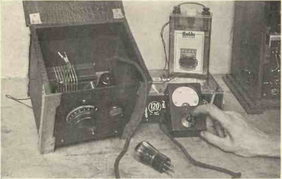
Fig. 12.—HOW TO TEST WHETHER THE CHOKE IS FAULTY.
