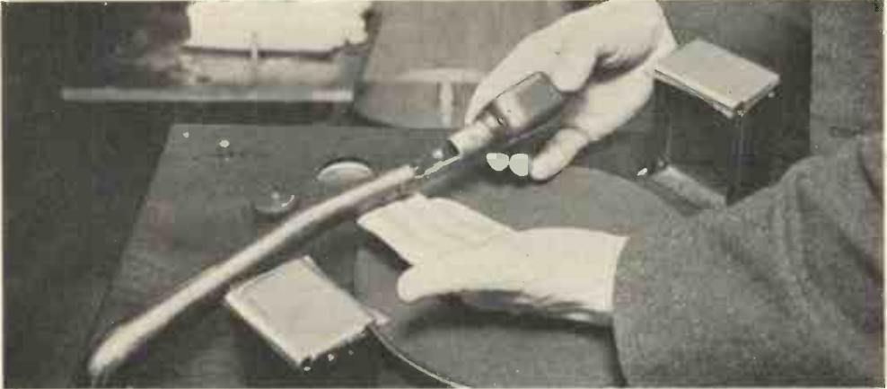
Fig. 9.—EXTRACTING THE PICK-UP HEAD OF AN H.M.V. RADIO-GRAMPHONE.
