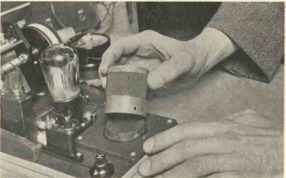
Fig. 3. —PLACING A COIL ON THE STAND. The stand is necessary so that each coil may occupy exactly the same position as the others.
