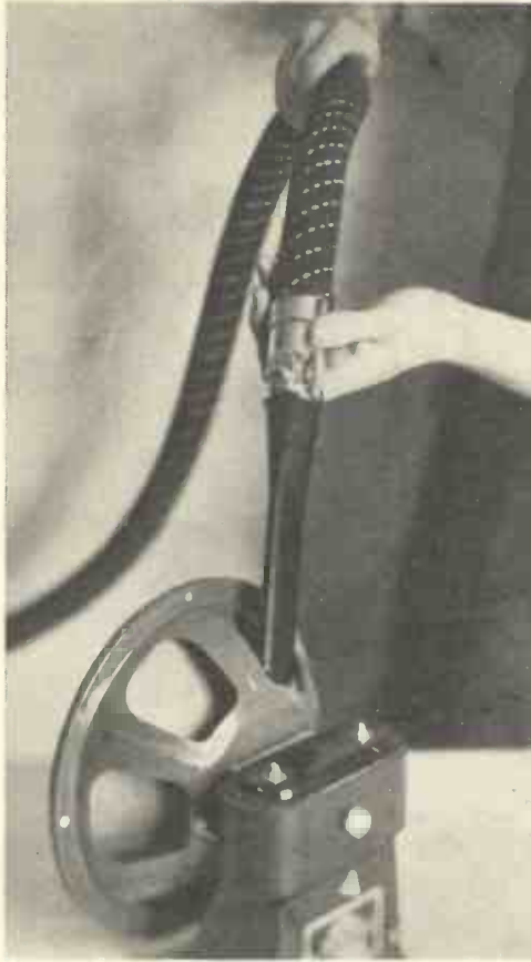
Fig. 6.—A TEMPORARY MEANS OF REMOVING DUST FROM THE GAP OF A MOVING COIL SPEAKER.
