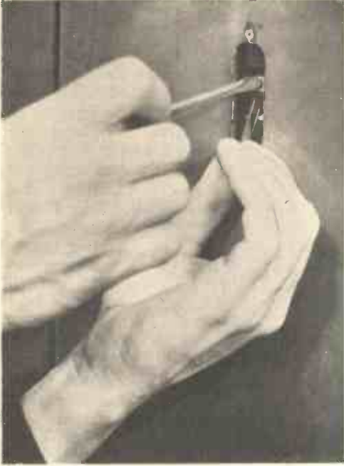
Fig. 3.—REMOVING THE LEVER OF THE WAVE-CHANGE SWITCH.
