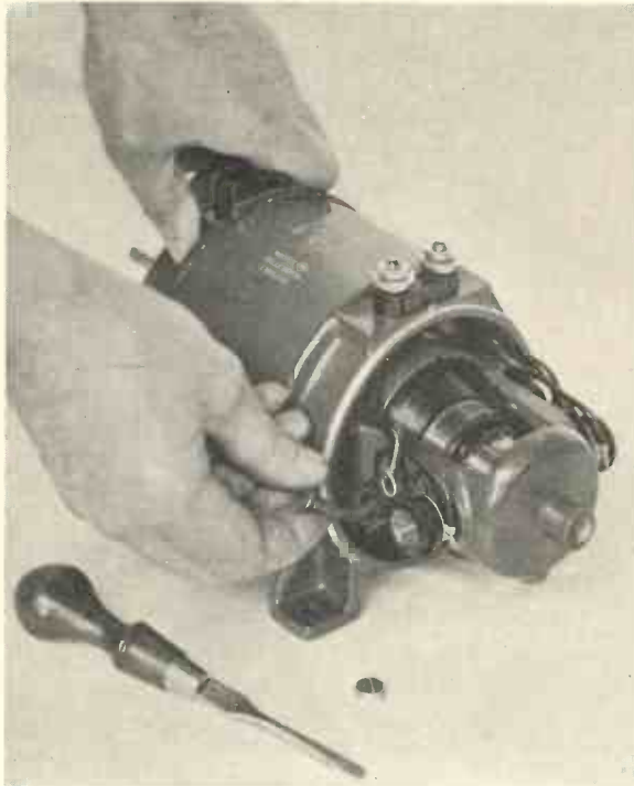
Fig. 15.—WITHDRAWING A BRUSH FROM A 100-WATT D.C. TO D.C. ROTARY TRANSFORMER.
