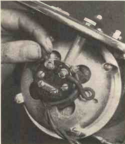
Fig. 28.—ADJUSTING THE GARRARD MOTOR FOR 100-130-VOLT SUPPLY.
