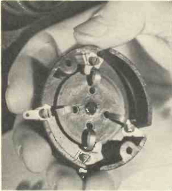
Fig. 4.—A POSSIBLE CAUSE OF TROUBLE. A broken spring in a valve holder can be the cause of many stoppages.
