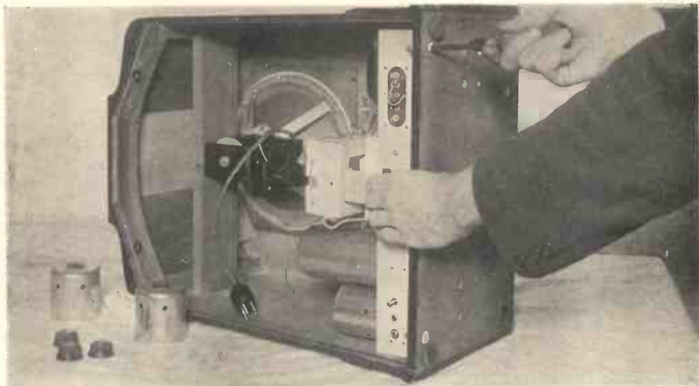
Fig. 31.—RELEASING THE CHASSIS SCREWS OF THE COLUMBIA 352 RECEIVER. This is done after taking off control knobs.
