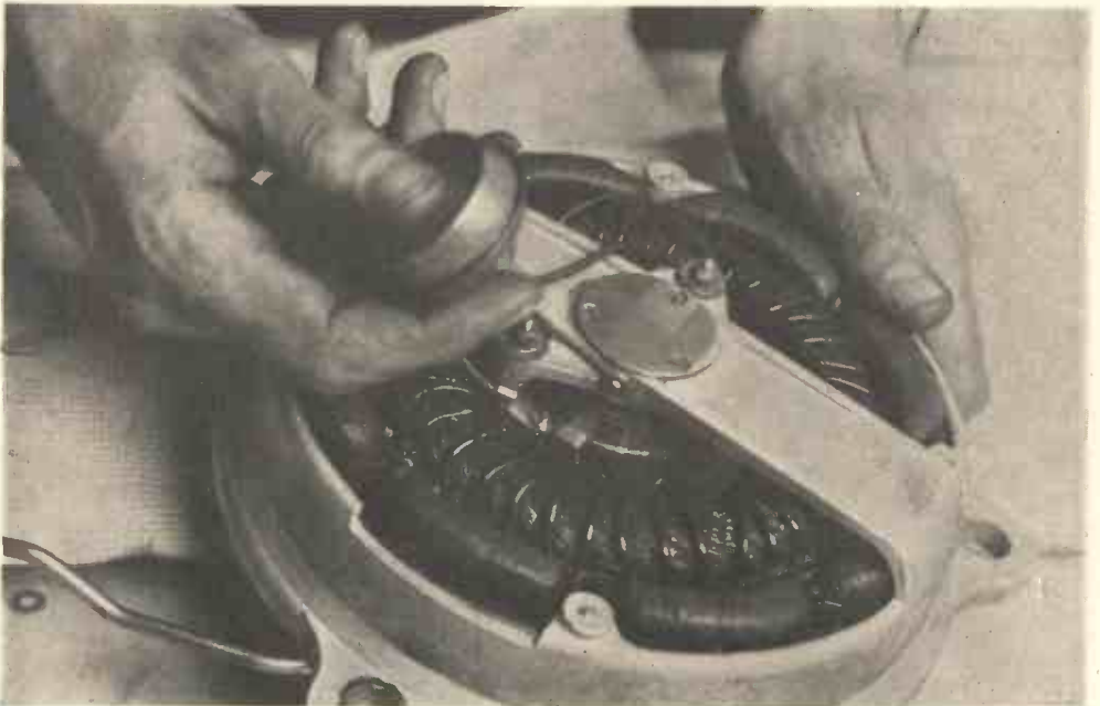
Fig. 20. —THIS SHOWS THE SPRING OIL NIPPLE FOR THE BOTTOM BEARING.
