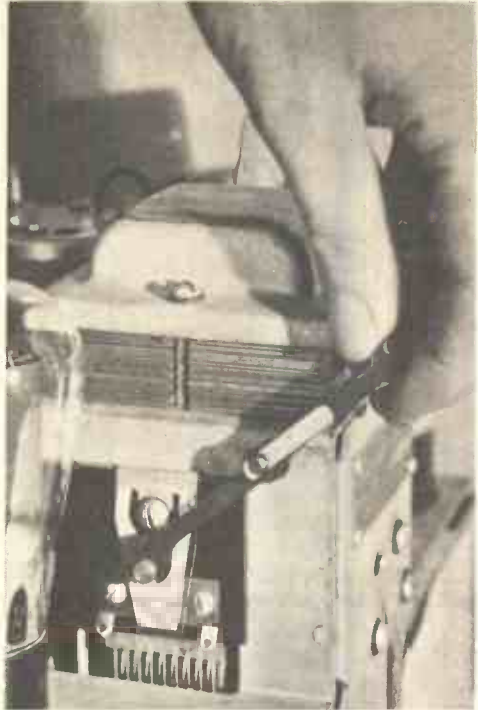
Fig. 5.—ADJUSTING THE ALIGNING CONDENSERS.
