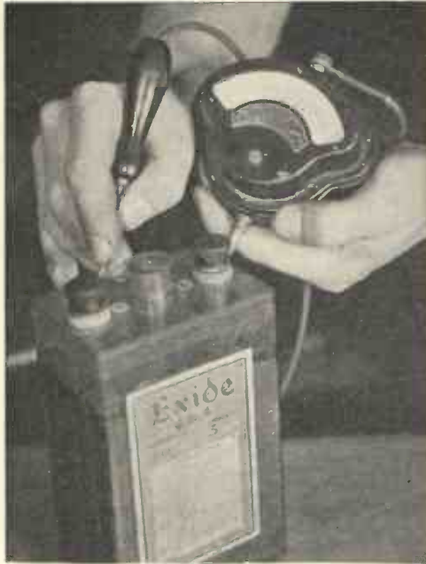
Fig. 4.—USING VOLTMETER TO TEST ACCUMULATOR.
