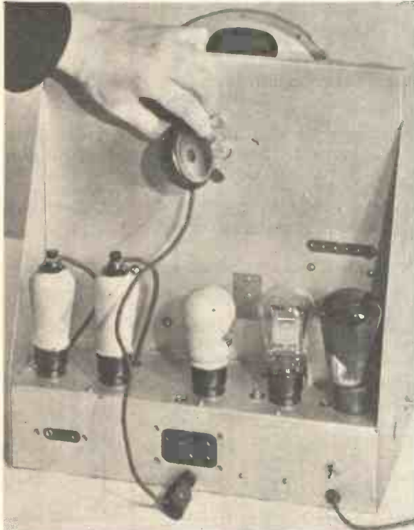
Fig. 21.—USING AN EAR-PIECE TO CHECK THE L.F. CIRCUITS.
