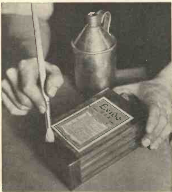
Fig. 15.—FINISHING OFF REPAIR TO LEAKY CONTAINER.
