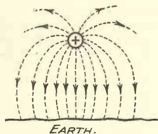
Fig. 12.—ELECTRIC FIELD PRODUCED WHEN A CHARGED SPHERICAL CONDUCTOR IS SUSPENDED IN AIR NEAR THE EARTH SURFACE.
