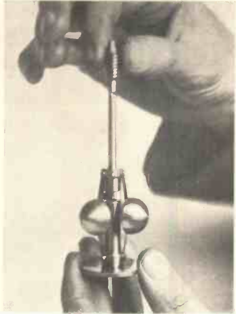
FIG. 4.—DETAILS OF THE GOVERNOR. Showing method of testing spindle.
