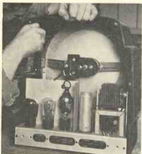
Fig. 25. —REMOVING RECEIVER FROM CABINET. SECOND STAGE.
