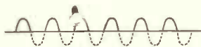
Fig. 12.—WHEN THE POINT A IN FIG. 11 IS NEGATIVE, A PULSATING CURRENT FLOWS DURING EACH HALF-CYCLE.
