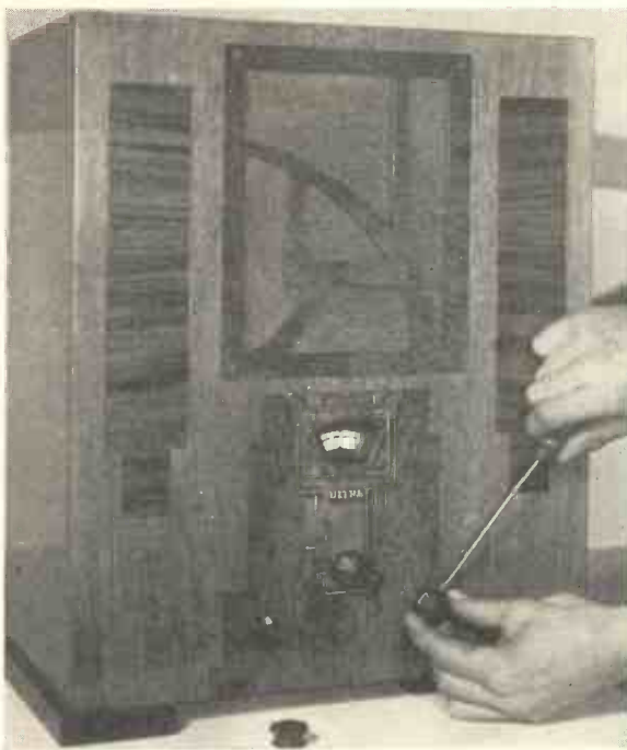
Fig. 1. —REMOVING THE THREE CONTROL KNOBS TO ALLOW THE CHASSIS TO BE WITHDRAWN FROM ITS CABINET.
