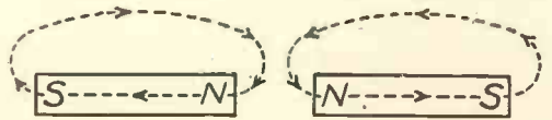
Fig. 5.—ANOTHER EXAMPLE OF FLOW OF LINES OF FORCE IN THE CASE OF LIKE POLES.
