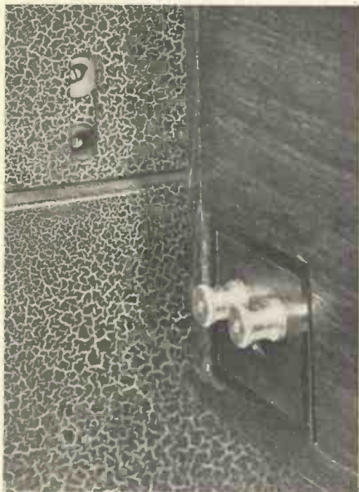
Fig. 8.—MAINS TERMINALS SHOULD BE SHROUDED.
