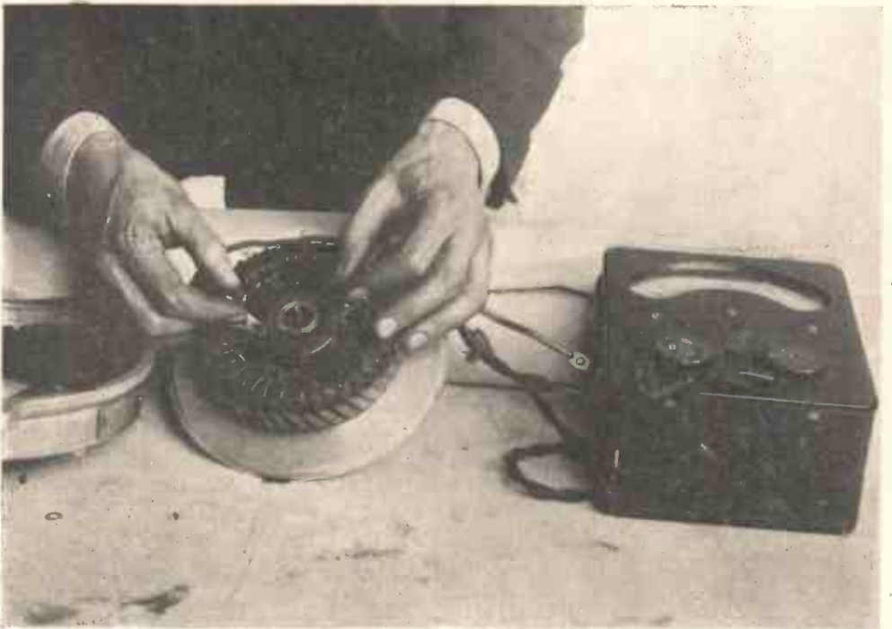
Fig. 22. —CHECKING UP THE CONNECTOR WINDINGS.
