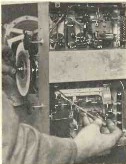
Fig. 4.—ADJUSTING THE PADDING CONDENSER. (ALL MAINS SUPER-HET.)
