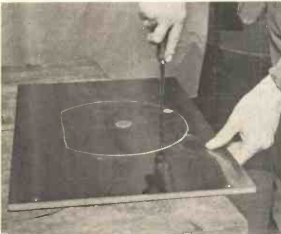
Fig. 8.—CUTTING THE HOLES IN THE FIVE-PLY-WOOD FOR THE LOUD SPEAKER DIAPHRAGMS.
