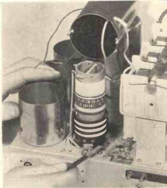
Fig. 38.—COIL COVER REMOVED FROM COLUMBIA 352, 603, AND 604 RECEIVERS. Showing switch contacts.
