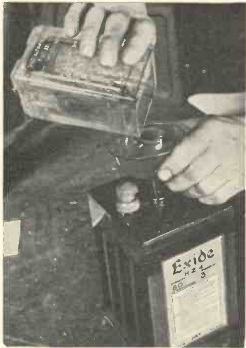
Fig. 5.—KEEP PLATES COVERED WITH ELECTROLYTE.
