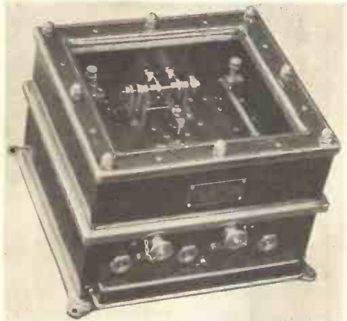
Fig. 4.—SELECTOR MECHANISM OF MARCONI AUTO ALARM APPARATUS.
