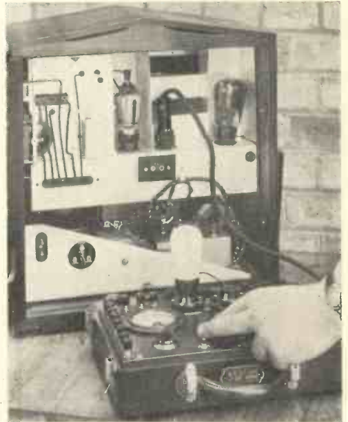
Fig. 18. —CHECKING VALVE OUTPUTS WHILE SET IS IN OPERATION.
