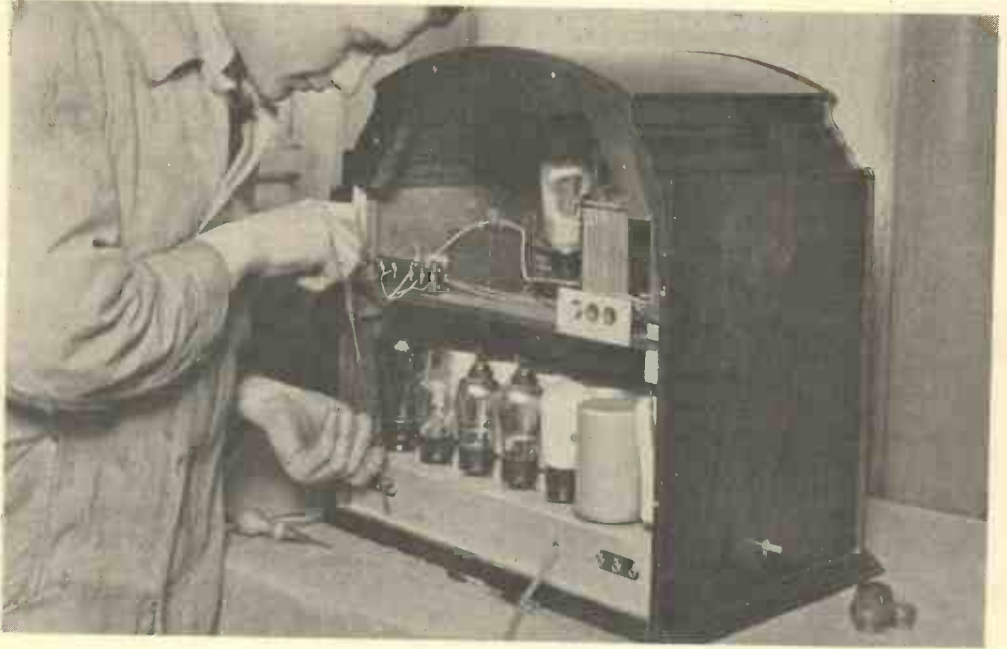
Fig. 5.—THE FOURTH OPERATION. Removing the three screws from chassis inside the cabinet.
