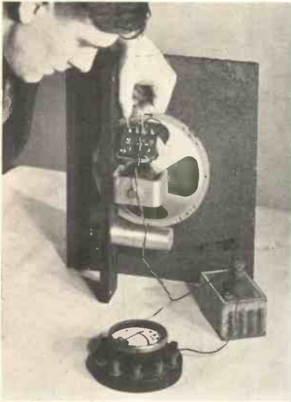
Fig. 6.—CHECKING THE RESISTANCE OF THE LOUD SPEAKER FIELD COIL.
