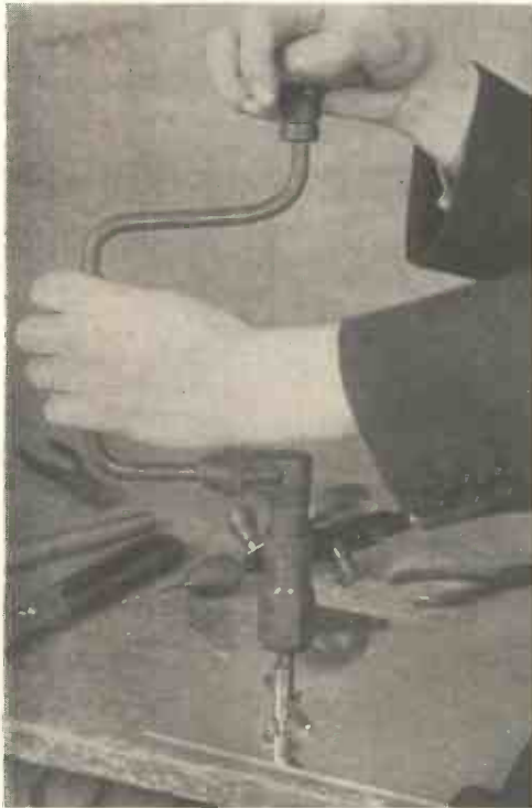
Fig. 16. —USING AN EXPANDING BIT FOR CUTTING LARGE DIAMETER HOLES.
