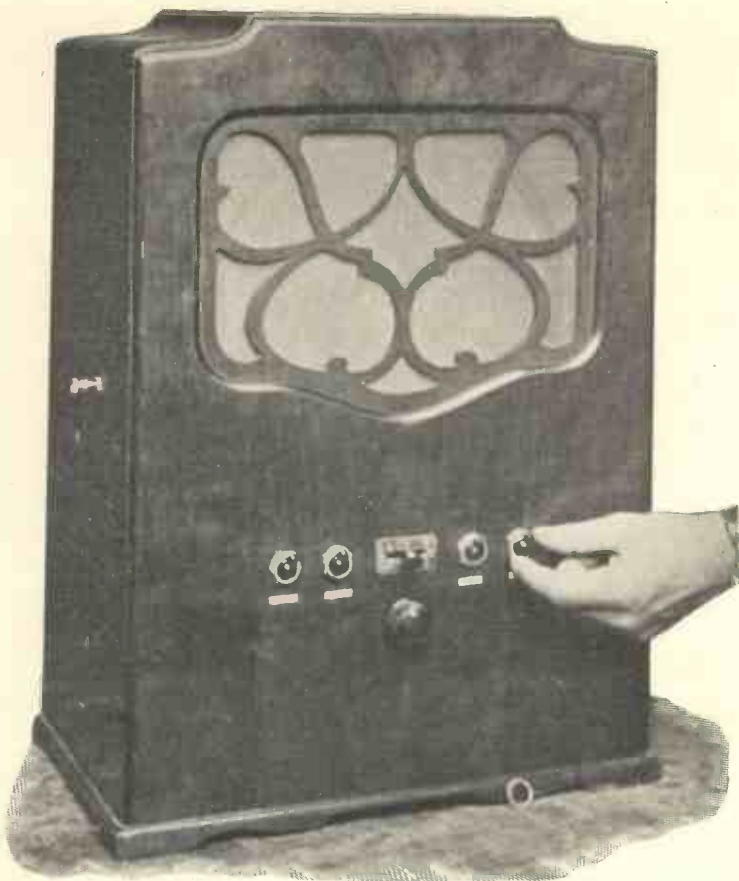
Fig. 7.—FIXING THE SWITCHES ON THE FRONT AFTER INSERTING THE BASEBOARD IN THE CABINET.
