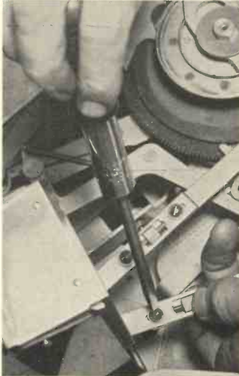
Fig. 28.—ADJUSTING WIDTH OF RECORD JAWS ON H.M.V. AUTOMATIC MECHANISM.
