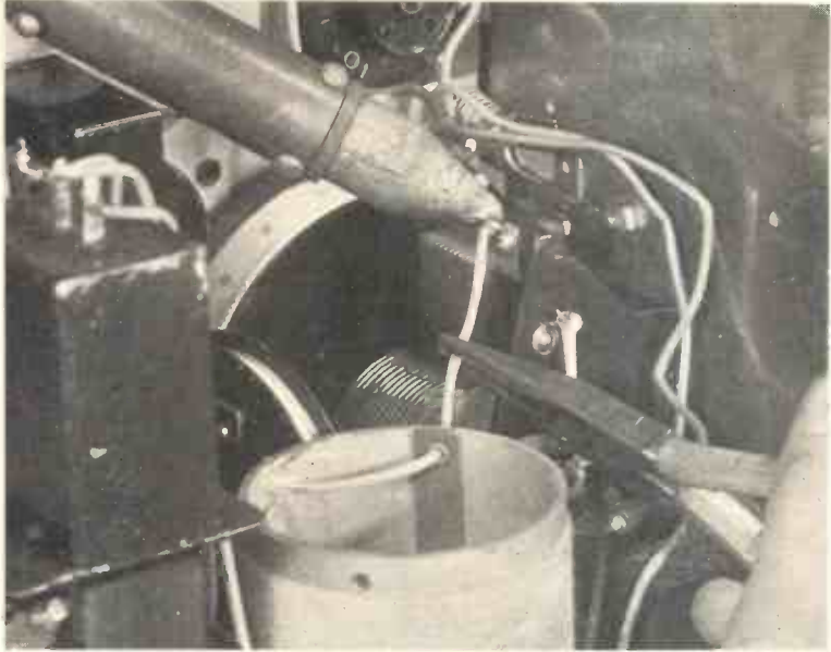
Fig. 16.—DISCONNECTING THE AERIAL CONDENSER OF THE COLUMBIA 307, 308 AND 310 RECEIVERS.
