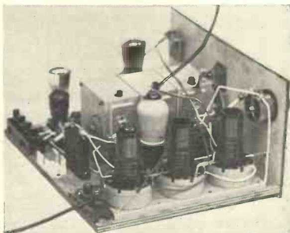
Fig. 5.—CUTTING OUT A SCREEN-GRID VALVE BY REMOVING THE AERIAL LEAD FROM ITS NORMAL TERMINAL AND CONNECTING IT TO THE ANODE TERMINAL OF THE S.G. VALVE.
