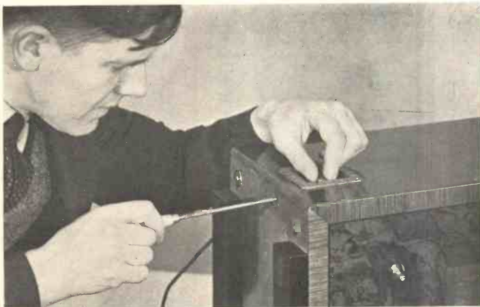
Fig. 16. —HOW THE SIDE CONTROL KNOBS ARE REMOVED.
