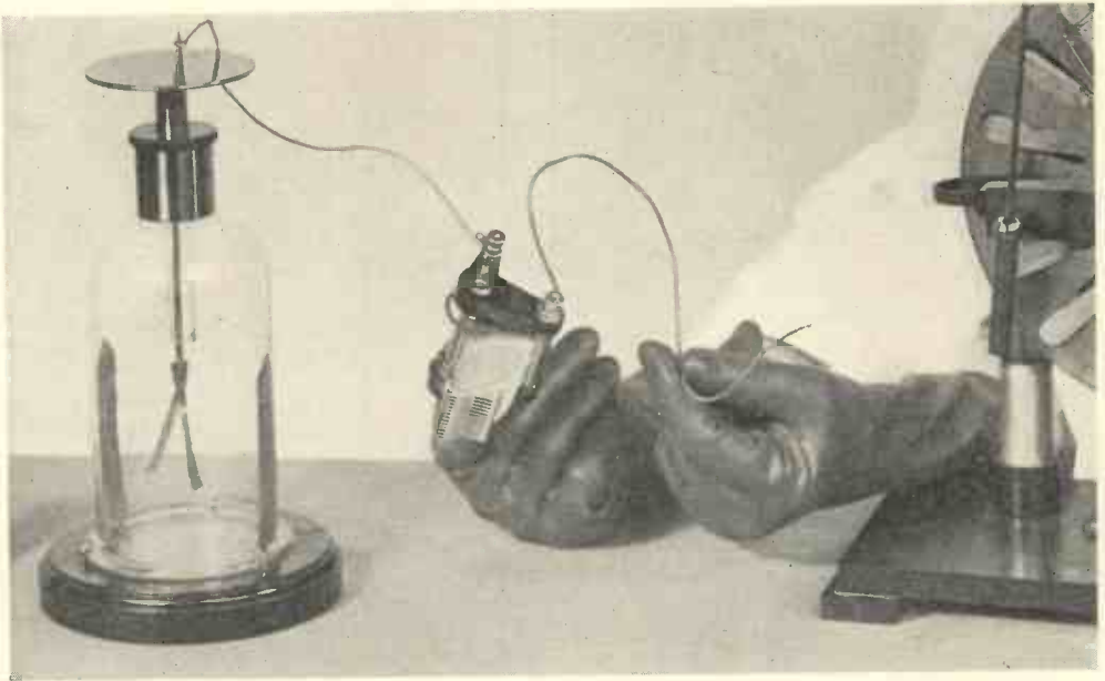
Fig. 15. —THE CONDENSER WILL RETAIN ITS CHARGE.
