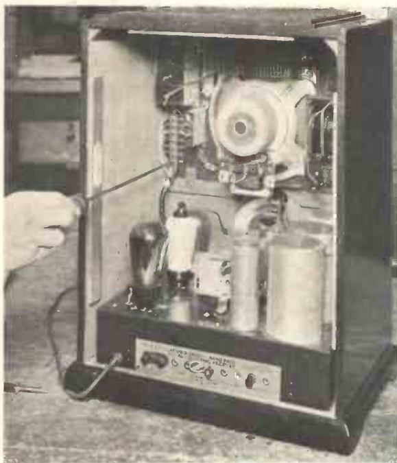
Fig. 4.—REMOVING THE TERMINAL STRIP.
