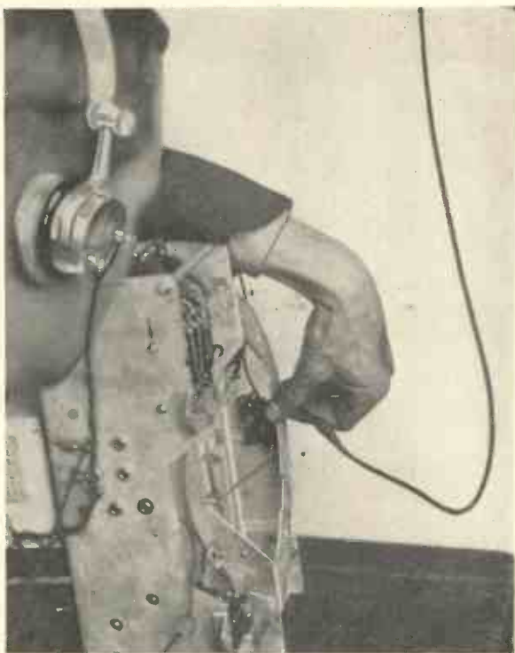
Fig. 7.—TESTING FOR FAULT ON THE SPINDLE WASHERS OF THE AERIAL TRIMMER CONDENSERS.
