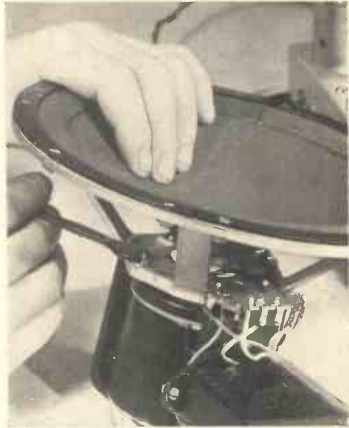
Fig. 45.—CENTERING THE LOUD SPEAKER CONE.
