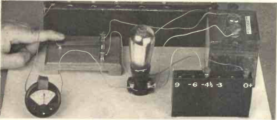
Fig. 25.—How THE ANODE CURRENT OF A POWER VALVE IS AFFECTED BY VARYING THE GRID VOLTAGE.
