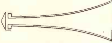
Fig. 6.—THE DIAPHRAGM IS HERE OF A LARGER DIAMETER THAN THE THROAT OF THE FLARE, WHICH NOW BECOMES A REAL HORN.
