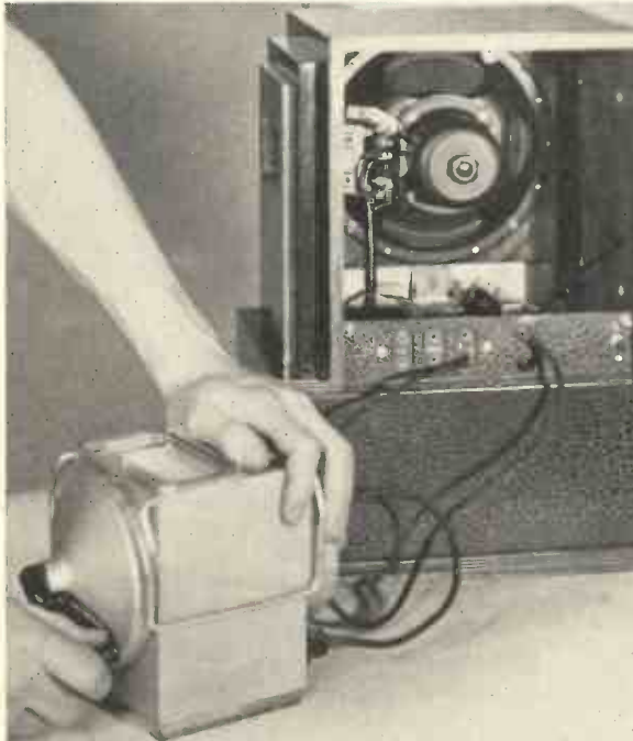
Fig. 10. —TESTING THE INSULATION RESISTANCE BETWEEN MAINS INPUT TERMINALS AND EARTH. (See also Fig. 9.)
