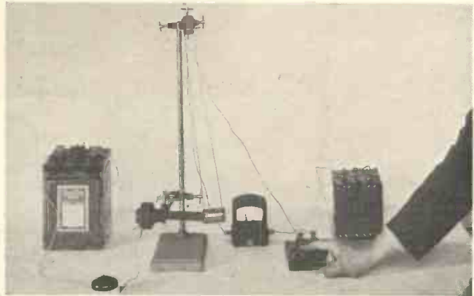
Fig. 3 (Above). —Note that the switch on the left has been closed and current is now flowing from the accumulator through the large coil turning the soft iron core into an electro-magnet. The switch in the moving coil circuit has been closed. Note the position of the coil.
