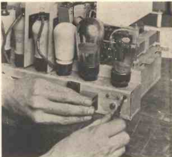
Fig. 2.—THIS SHOWS THE METHOD OF SETTING THE AERIAL TRIMMER.
