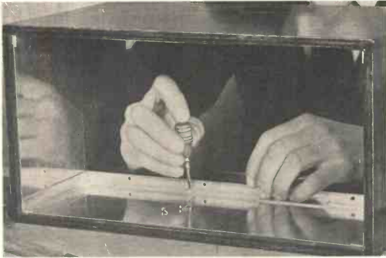
Fig. 7.—FITTING THE INTERNAL SHIELDS TO THE CABINET.
