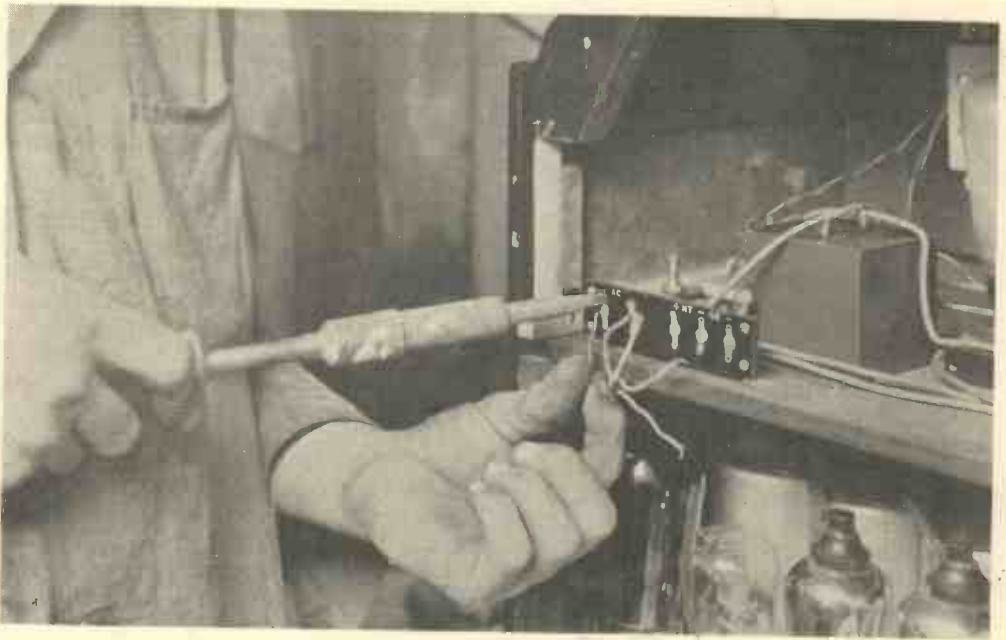
Fig. 6.—THE FIFTH OPERATION. Unsoldering the leads from the output board.
