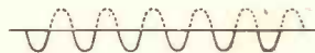
Fig. 14.—WHEN THE POINT A IN FIG. 13 IS POSITIVE, THE GRID WILL BECOME POSITIVE AND A CURRENT WILL FLOW THROUGH THE VALVE.
