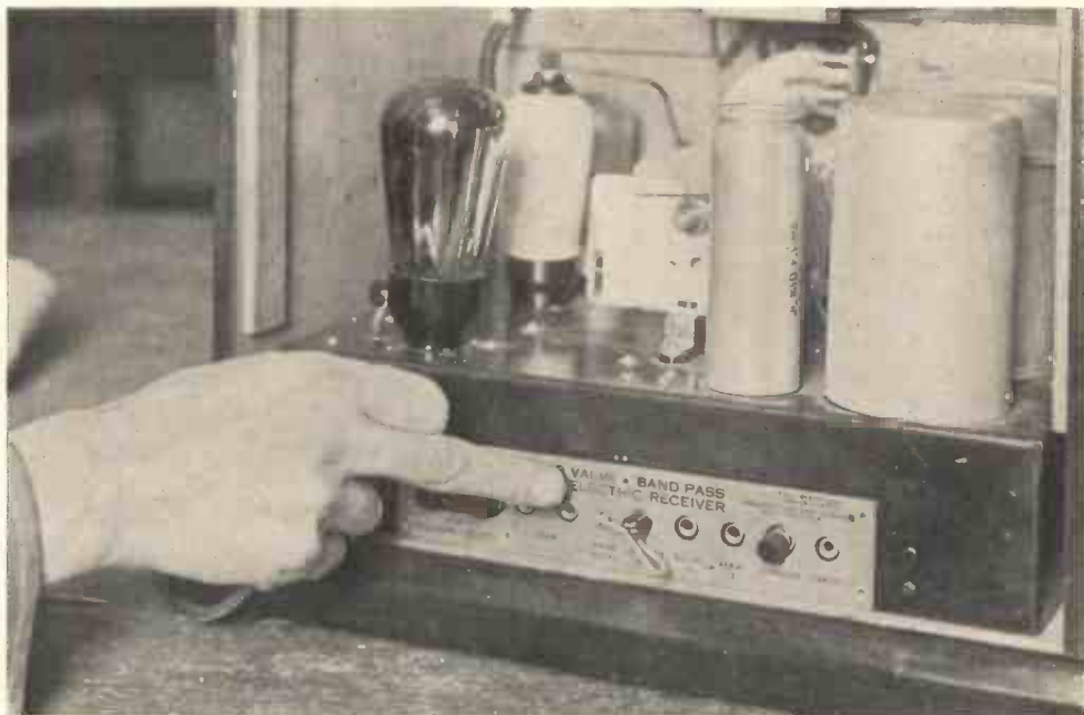
Fig. 13. —CHECKING UP THE DETECTOR AND AMPLIFYING STAGES OF THE RECEIVER.
