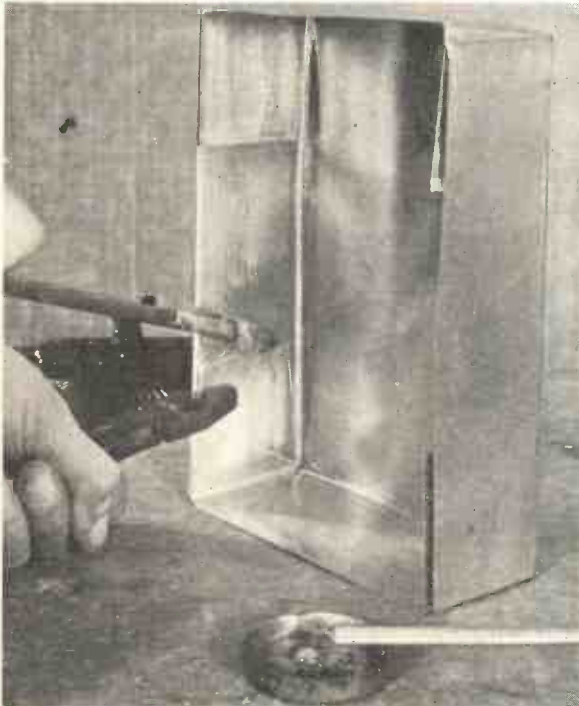
Fig. 8.—THE CORNERS ARE HELD WITH PLIERS WHEN SOLDERING THE LUGS.
