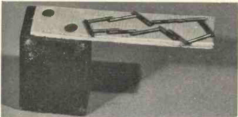
Fig. 18.—WHAT HAPPENS WHEN A PIECE OF IRON IS MAGNETISED.
