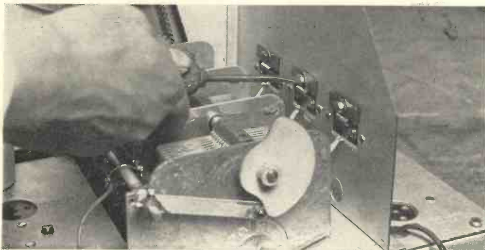
Fig. 16. —HOW TO ADJUST THE MEDIUM WAVE TRIMMERS TO OBTAIN CORRECT GAUGING.
