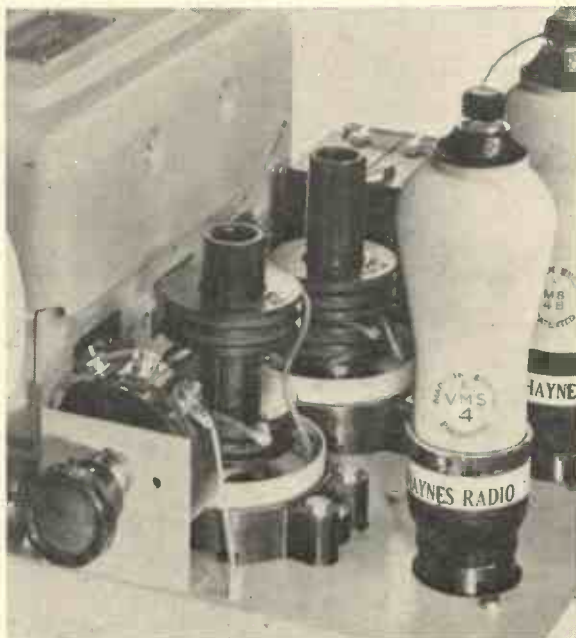
Fig. 4.—THE INTERMEDIATE AMPLIFIER COUPLINGS WITH TUNING COVERS REMOVED.
