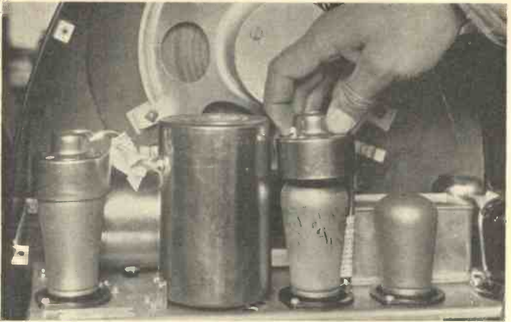
Fig. 10. —HOW TO FIT THE COPPER SCREENING CAPS ON THE SCREEN-GRID VALVES.
