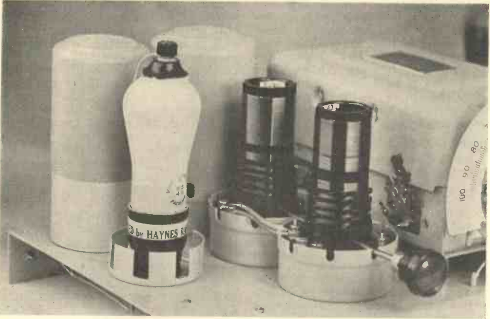
Fig. 2. —INPUT FILTER COILS USING INDUCTIVE AND CAPACITY COUPLINGS.
