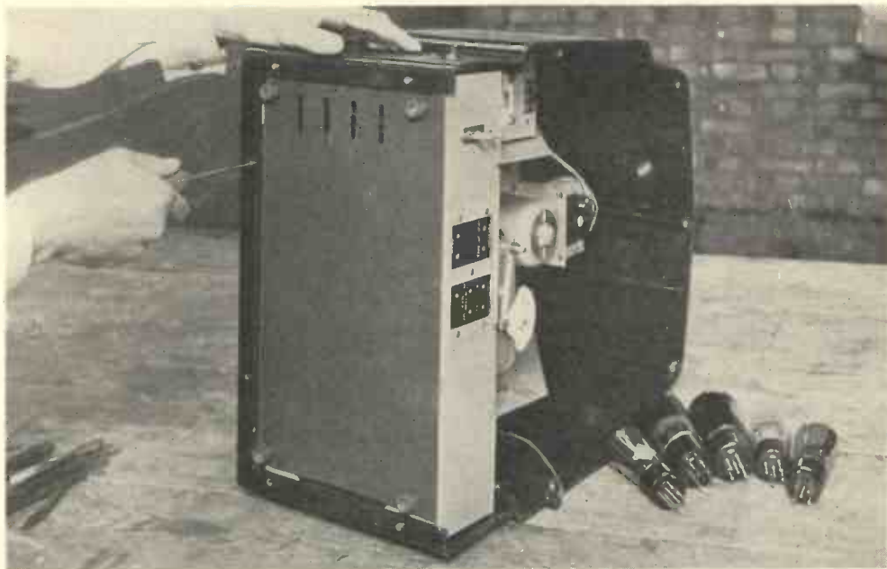
Fig. 1.—How to remove the R.S.3 Receiver from the Cabinet, First Operation.
