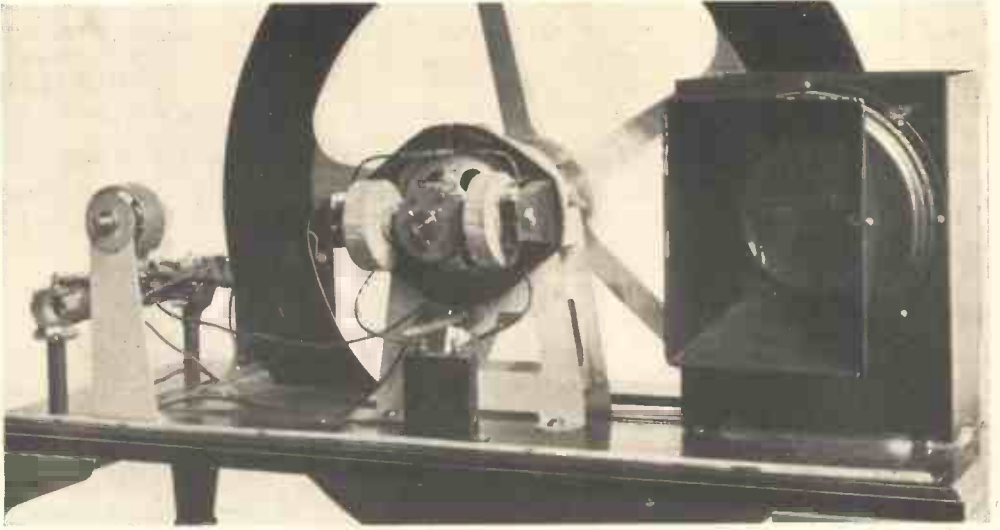
Fig. 4.—THE "TELEVISOR" WITH CASE REMOVED.
