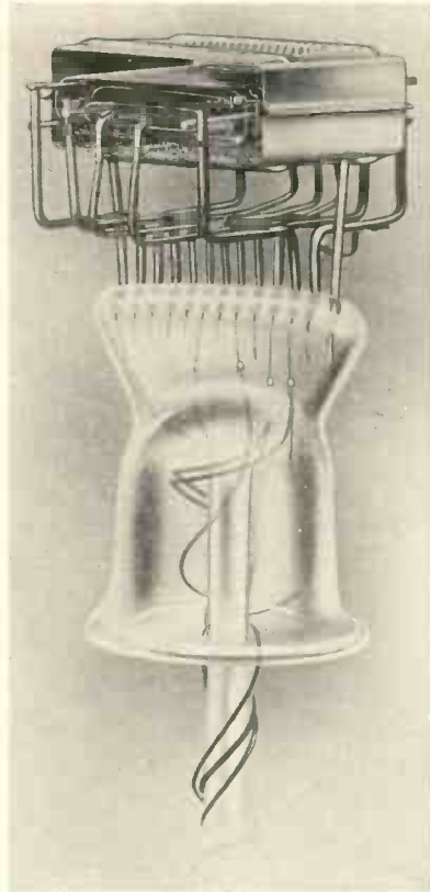
Fig. 5.—THE COMPLETE FOOT ASSEMBLY READY FOR SEALING IN BULB.
