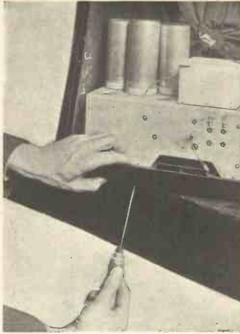
Fig. 10.—REMOVING THE CHASSIS SECURING SCREWS BY RESTING THE BASE OF THE CABINET OVER THE EDGE OF A TABLE.
