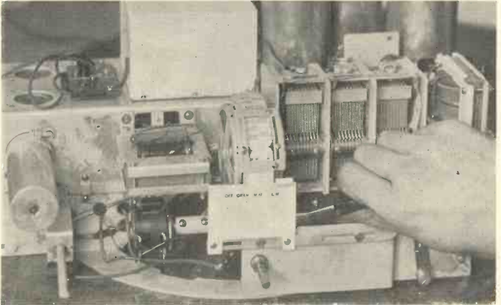
Fig. 21.—BENDING BACK THE WAVECHANGE INDICATOR SCALE TO CLEAR ESCUTCHEON.
