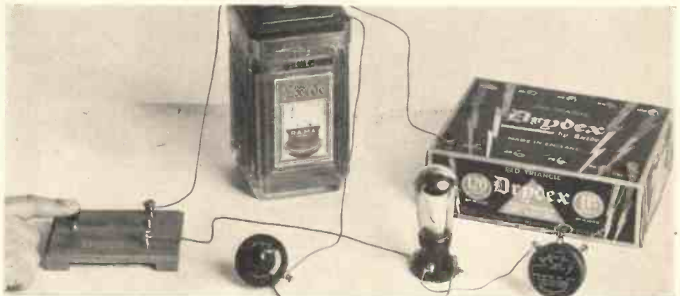
Fig. 6.—EXPERIMENT SHOWING HOW ANODE CURRENT VARIES WITH FILAMENT CURRENT. The filament current is at full strength, and the anode current is 30 m.a.
