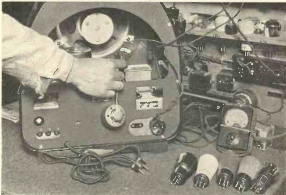
Fig. 1. —MAKING A LOW VOLTAGE CIRCUIT TEST ON A PHILIPS 830A RECEIVER.
