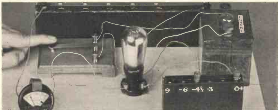
Fig. 23.—HOW THE ANODE CURRENT OF A POWER VALVE IS AFFECTED BY VARYING THE GRID VOLTAGE.
