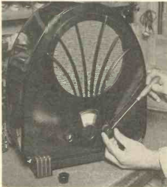
Fig. 3.—SECOND STAGE. Removing the fixing screws.
