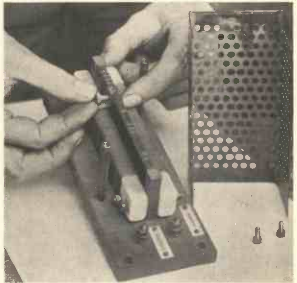
Fig. 12.—ADJUSTING THE RESISTOR OF THE TYPE 82 MOTOR FOR THE VOLTAGE OF THE MAINS.
