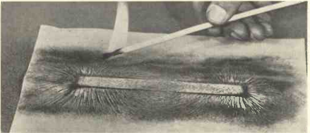
Fig. 5.— DEMONSTRATING MAGNETIC FIELDS. Use a taper to melt the paraffin, thus fixing the filings in position.
