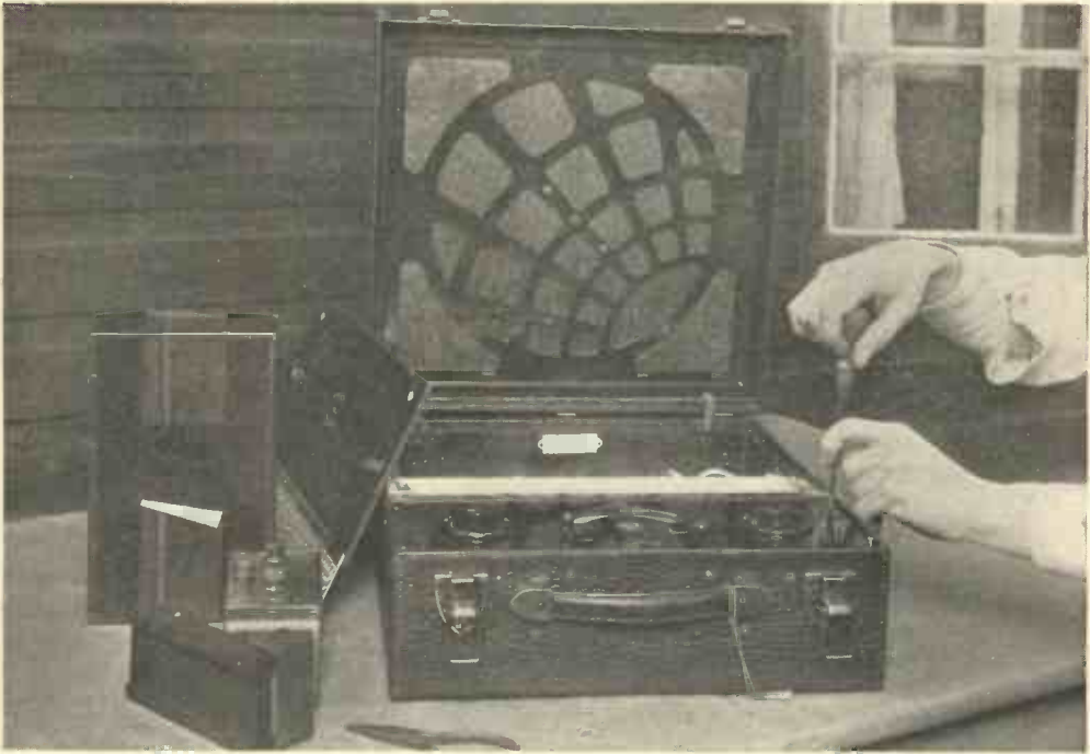
Fig. 1.—How to REMOVE CHASSIS OF THE DUPLEX FOUR SUITCASE ("S") TYPE. FIRST OPERATION. After removing battery panel in the usual way, take out both high tension battery and accumulator. Remove the eight raised head screws from the ebonite of the tuning panel.
