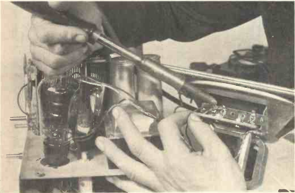
Fig. 11. —DETACHING LOUD SPEAKER FROM THE CHASSIS.
