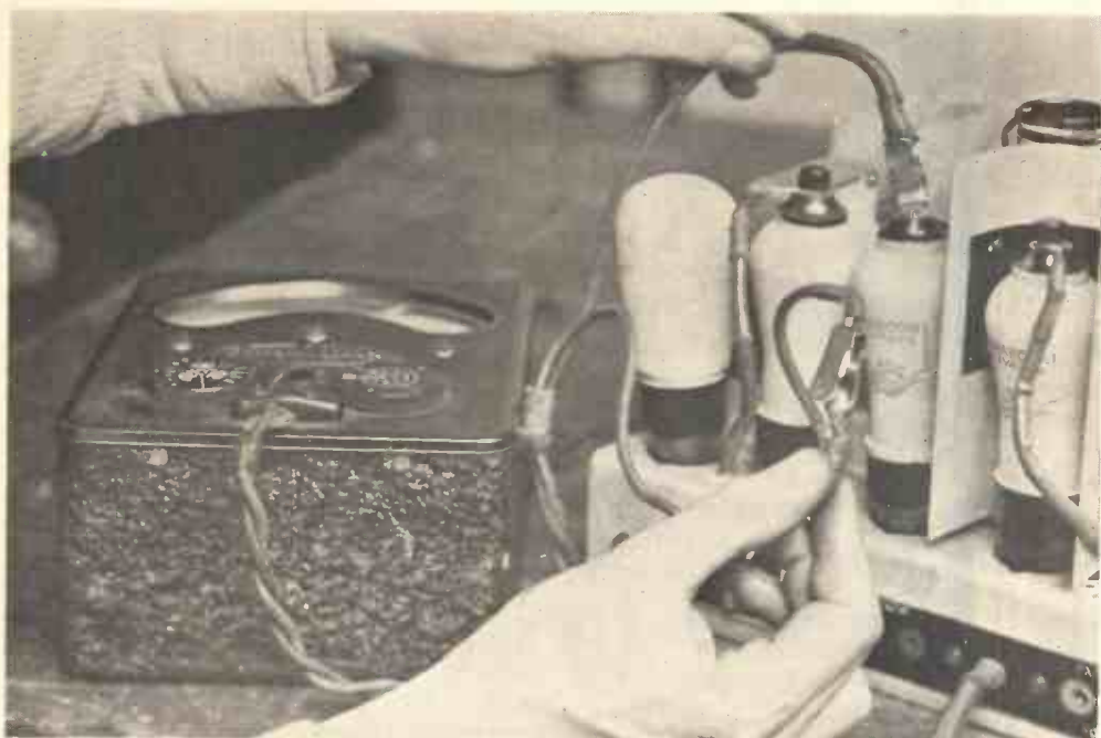
Fig. 4.—MEASURING THE EMISSION OF THE SCREENED-GRID VALVE OF MARCONI 535.
