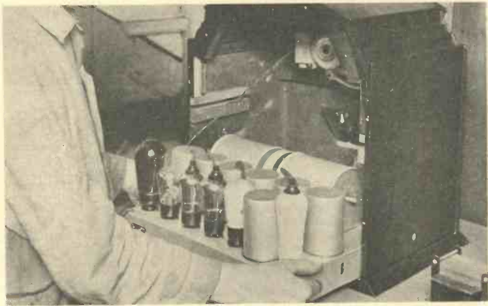
Fig. 11. —WITHDRAWING THE RECEIVER CHASSIS.
