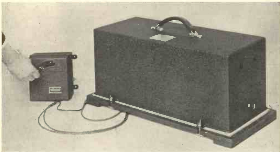
Fig. 12.—OPERATING THE STARTER TO START A LARGE D.C. TO A.C. ROTARY TRANSFORMER.
