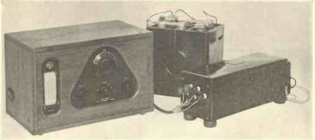
Fig. 2.—AN M-L ANODE CONVERTER CONNECTED TO A MODERN SHORT-WAVE RECEIVER (Rotax Ltd.).
