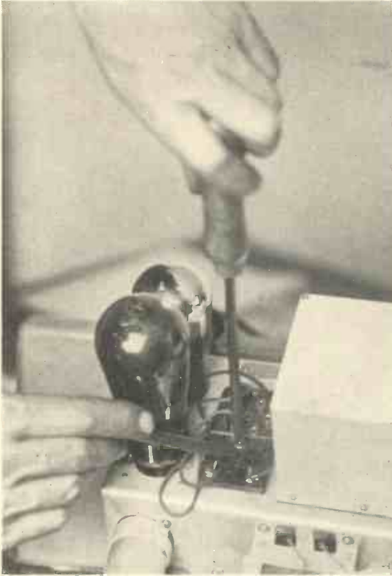
Fig. 16.—ADJUSTING THE HUM ADJUSTER.
