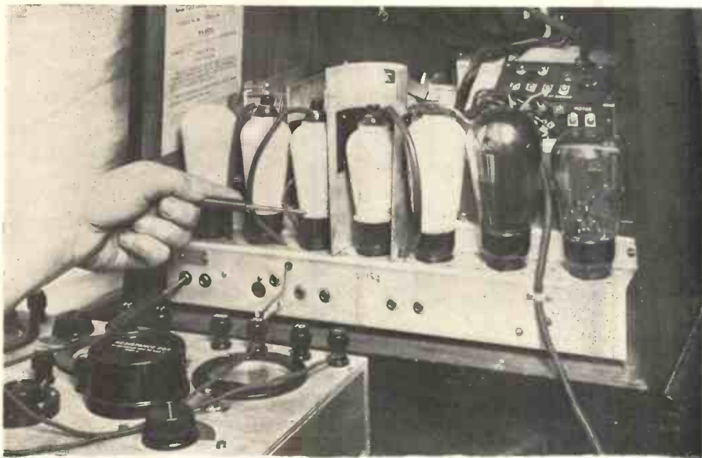
Fig. 1.—A QUICK METHOD OF TESTING THE GRID BIAS VOLTAGES OF THE METALLISED VALVES IN THE MARCONIPHONE MODEL 256 SUPERHETERODYNE.
