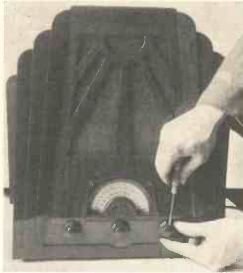
Fig. 1. —REMOVING OF CHASSIS FROM CABINET. FIRST STAGE.
