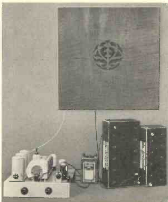
Fig. 1.—THE OPTIMUM THREE VALVE RECEIVER WITH BATTERIES AND LOUD SPEAKER CONNECTED READY FOR TEST.
