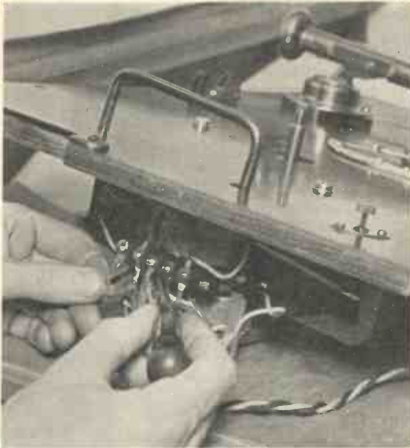
Fig. 15.—ADJUSTING THE MOTOR FOR VOLTAGE OF SUPPLY.
