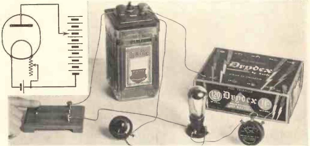
Fig. 4.—EXPERIMENT SHOWING HOW ANODE CURRENT VARIES WITH FILAMENT CURRENT. Here the filament current is only just on, and the anode current is 2 m.a. Fig. 4A (inset) shows the connections diagrammatically.
