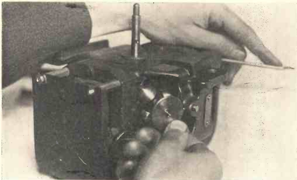
Fig. 10.—TAKING OUT THE GOVERNOR FROM THE MOTOR.
