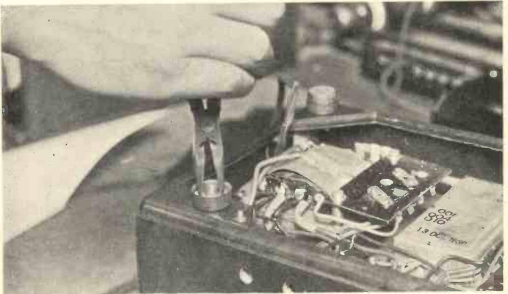
Fig. 22. —HOW TO REMOVE THE SEALS.
