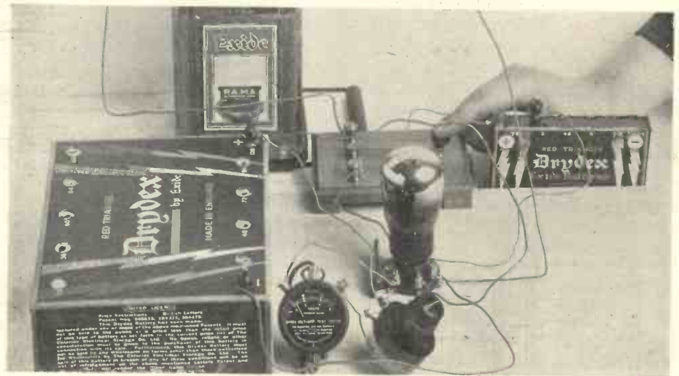
Fig. 2.—EFFECT OF VARYING RESISTANCE IN ANODE CIRCUIT OF PENTODE. With 25,000 ohms additional resistance in anode circuit, anode current equal 4 milliamps.
