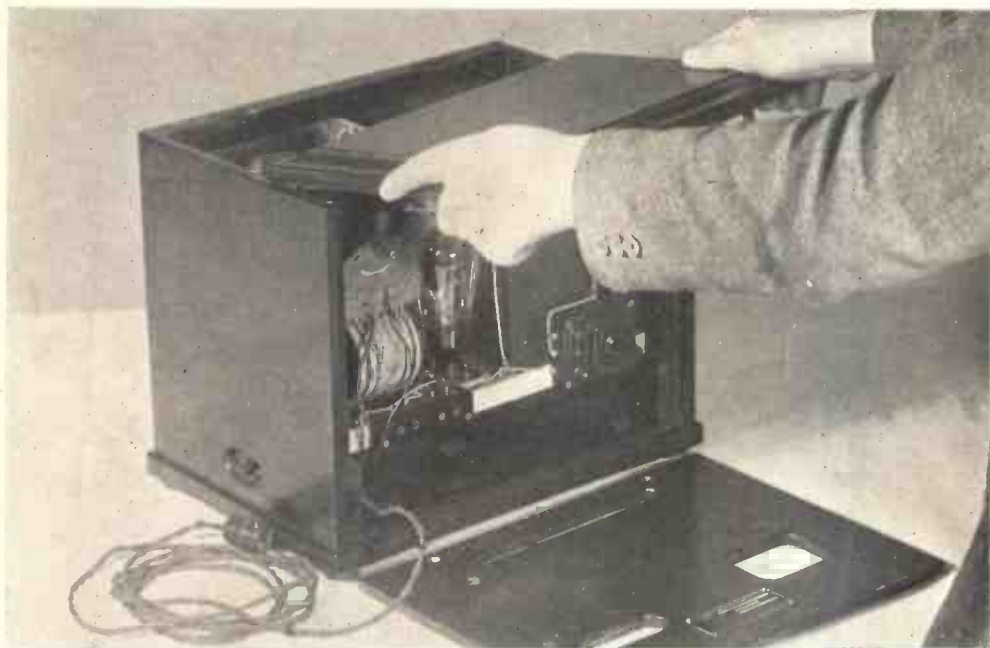
Fig. 1. —DISMANTLING THE COLUMBIA 307 RECEIVER.
