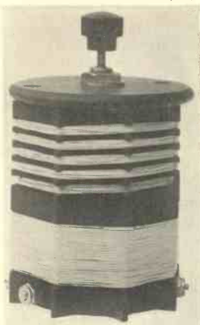
Fig. 1.—A COMPLETED COIL WITH WAVECHANGE SWITCH READY FOR MOUNTING ON THE PANEL OF A SET. Full instructions for winding such a coil are given in Figs. 21 to 27.
