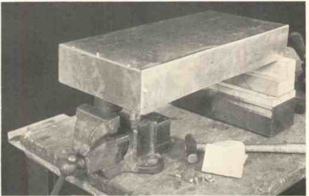
Fig. 12. —HOW THE WORK IS HELD DURING RIVETING.
