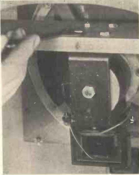
Fig. 44.—How to REMOVE THE LOUD SPEAKER FROM THE CABINET OF THE COLUMBIA 352 RECEIVER.
