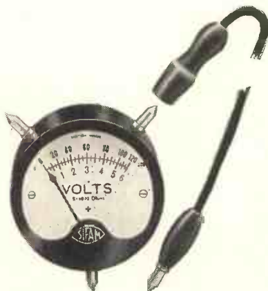
Fig. 6.—A VOLTMETER HAVING TWO SCALES, ONE FROM 0-6 VOLTS AND THE OTHER 0-120 VOLTS.
