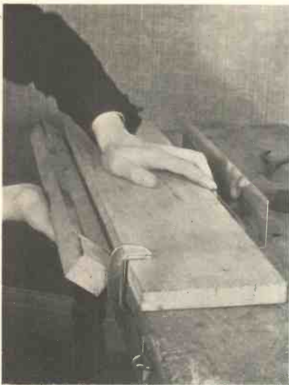
Fig. 10.—BENDING THE ALUMINIUM SHEET WITH A BLOCK SCREWED TO THE BENCH.
