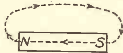
Fig. 1.—SHOWING HOW IN AN ORDINARY MAGNET THE LINES OF FORCE START AT THE NORTH POLE AND TERMINATE AT THE SOUTH POLE.
