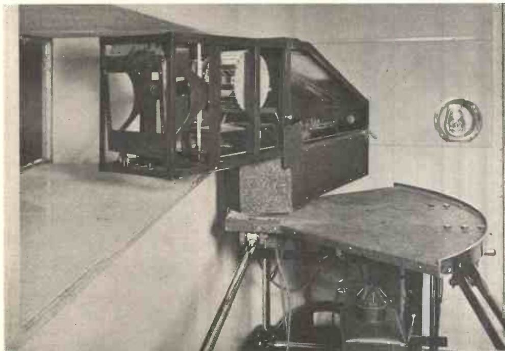
Fig. 1. —THE TELEVISION APPARATUS USED BY THE BRITISH BROADCASTING CORPORATION. The cover of the apparatus has been removed to show the inside arrangement.
