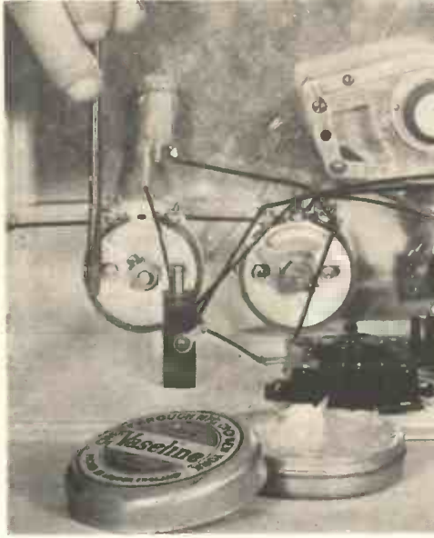
Fig. 17.—THE VASELINE ON THE ATTENUATOR WILL ENSURE SMOOTH AND SILENT OPERATION.
