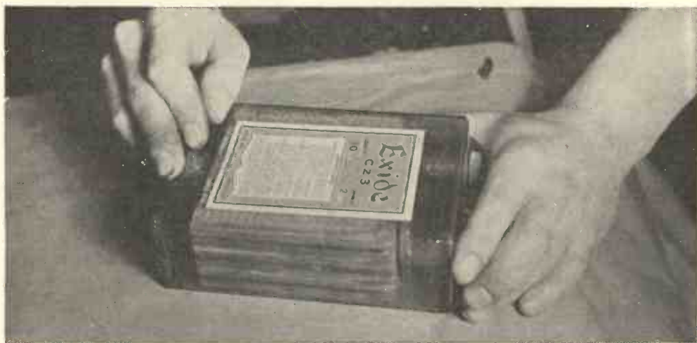
Fig. 13.—CURING LEAKY CELLULOID CONTAINER.
