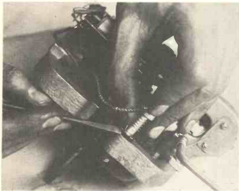
Fig. 4.—ADJUSTING THE BRUSH PRESSURE OF THE H.M.V. TYPE 25 MOTOR.
