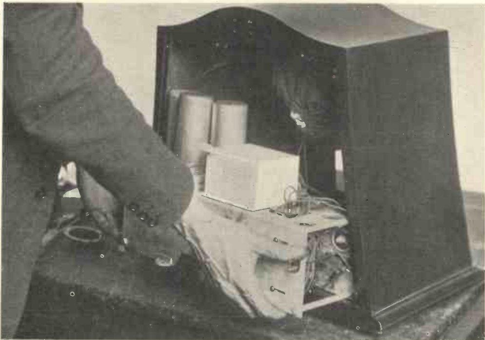
Fig. 14. —THE RIGHT WAY TO LIFT OUT THE CHASSIS.
