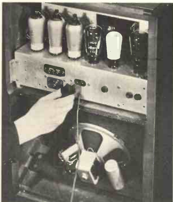
Fig. 1.—FITTING AN UNWIRED PLUG TO THE SAFETY SOCKETS OF THE KOLSTER-BRANDES RECEIVER MODELS 285 AND 286.
