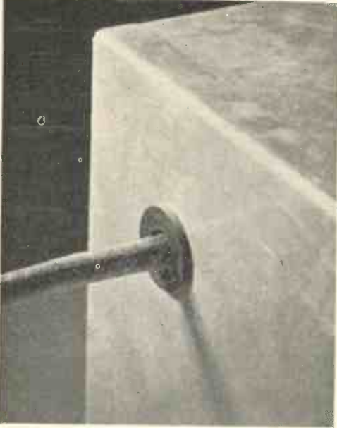
Fig. 2. —THE PROPER WAY TO MAKE A HOLE IN A METAL CASE.
