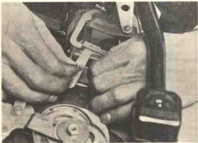
Fig. 13.—ADJUSTING THE RATCHET PLATE SPRING.
