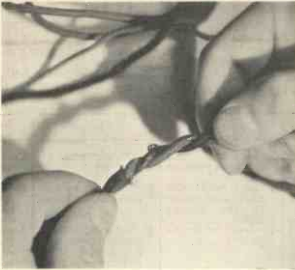
Fig. 2.—TESTING OLD FLEX FOR BREAKS. This is done by bending it inch by inch as shown.
