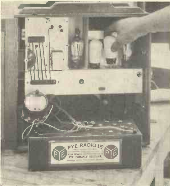
Fig. 20.—TESTING EMISSION OF VALVES ON PYE "Q" RECEIVER.
