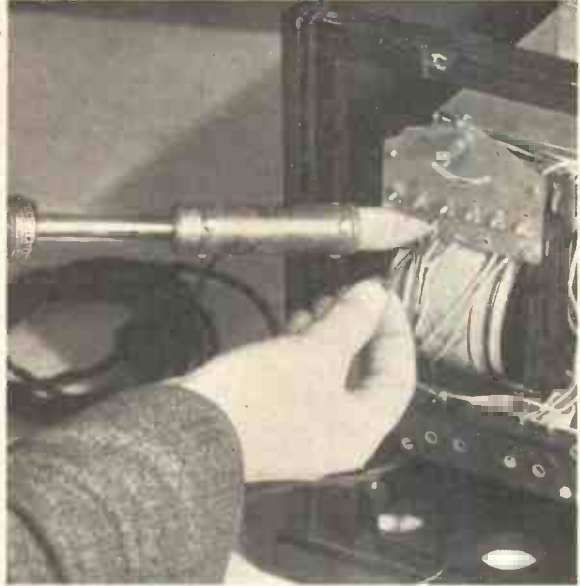
Fig. 4.—How the Mains Switch Lead is Removed.
