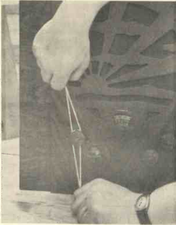
Fig. 29.—HOW TO REMOVE THE KNOBS OF THE "K" AND "G" MODELS.
