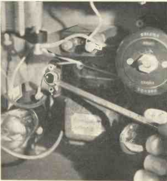
Fig. 5.—WHAT TO DO IF THE VALVES DO NOT LIGHT. If the valves fail to light make sure that the fuse bulb is not broken.
