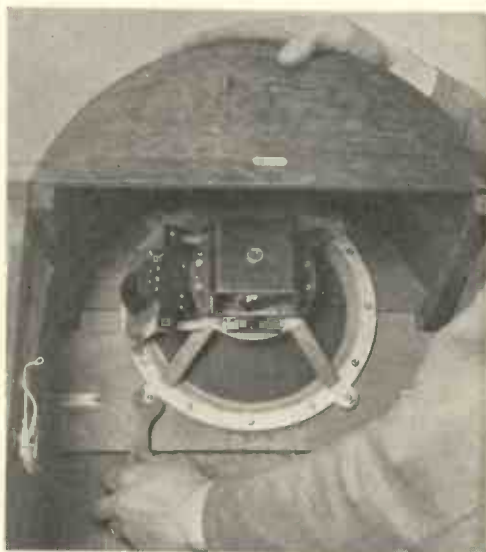
Fig. 13.—TIGHTENING UP THE BAFFLE BOARD.
