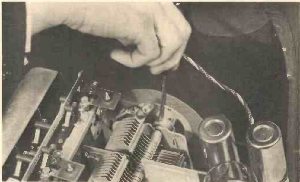
Fig. 6. —LOOSENING THE GRUB SCREW RELEASES THE DIAL FROM THE MAIN CONDENSER SPINDLE.
