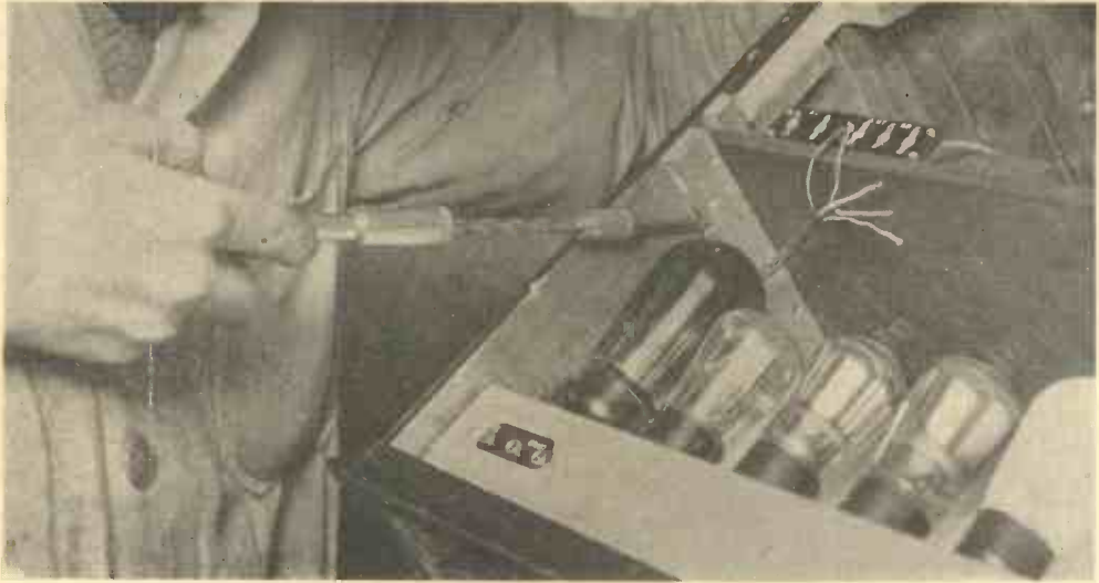
Fig. 7.—THE SIXTH OPERATION. Removing the screws which hold the power pack to the baseboard.
