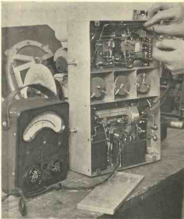
Fig. 20.—MAKING A CONTINUITY TEST.
