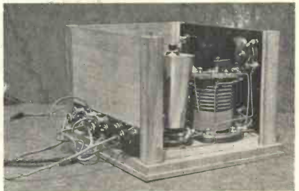
Fig. 10.—THIS SHOWS HOW THE LOOSE PANELS ARE SLID INTO THE GROOVES.
