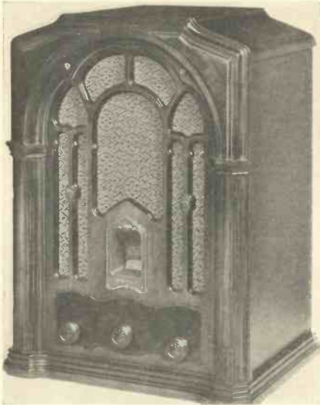
Fig. 14.—RCA VICTOR MODEL R.74. A ten-valve superheterodyne receiver.
