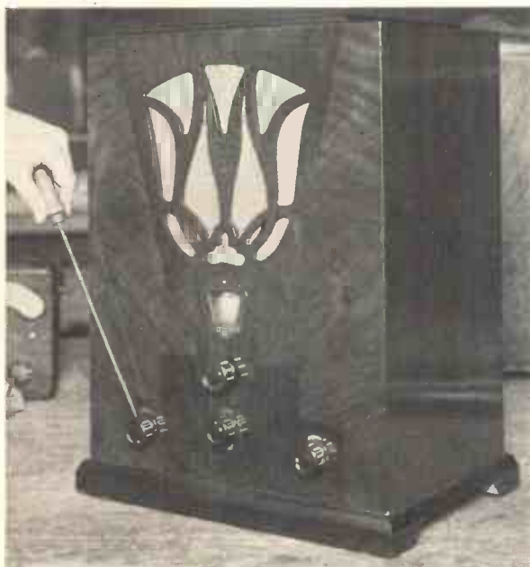
Fig. 9.—HOW TO WITHDRAW THE CHASSIS AND POWER PACK FROM THE CABINET.
