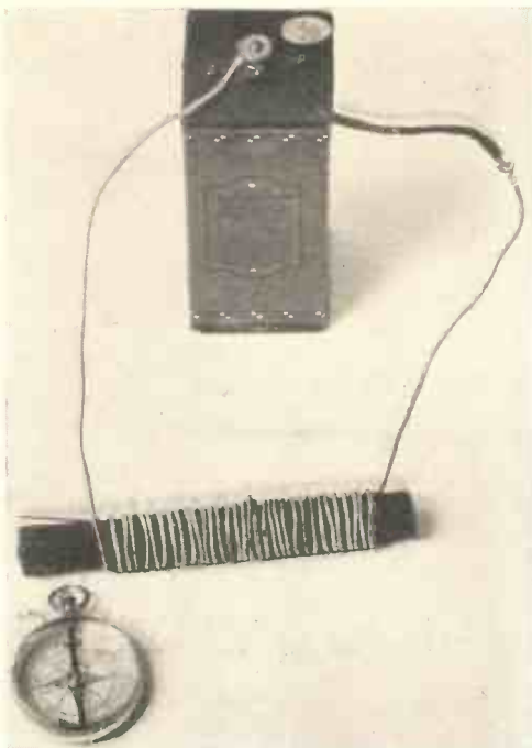
Fig. 5A.—WORK IT OUT YOURSELF. Remembering that the centre terminal of battery is positive.
