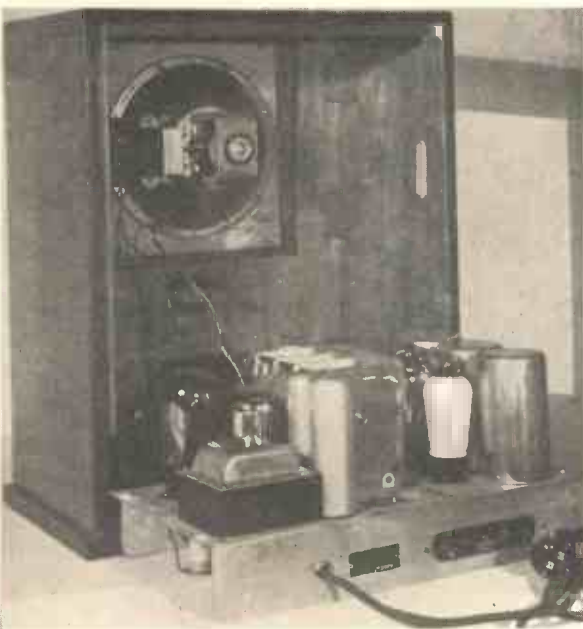
Fig. 4.—THE CHASSIS CAN BE WITHDRAWN WITHOUT DISCONNECTING THE LOUD SPEAKER.
