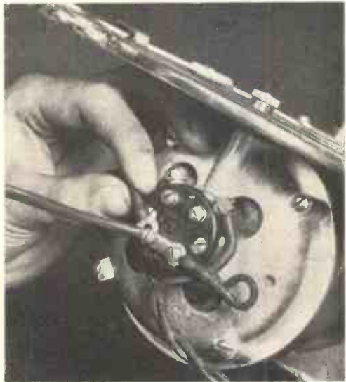
Fig. 29.—ADJUSTING THE GARRARD MOTOR FOR 200-250-VOLT SUPPLY.
