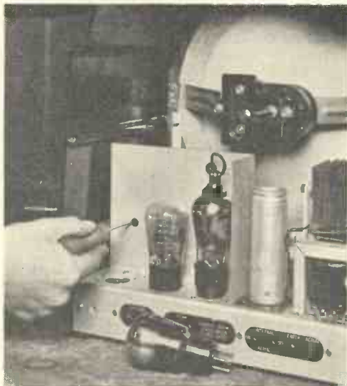
Fig. 26. —REMOVING RECEIVER FROM CABINET. THIRD STAGE.
