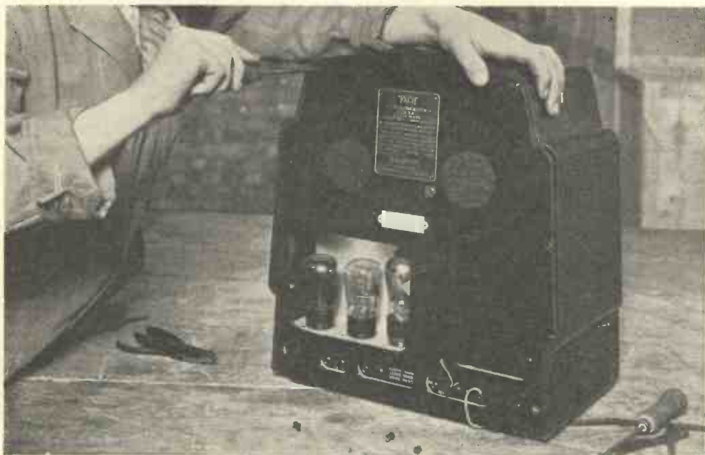
Fig. 24. —REMOVING THE R.S.2 RECEIVER FROM THE CABINET.
