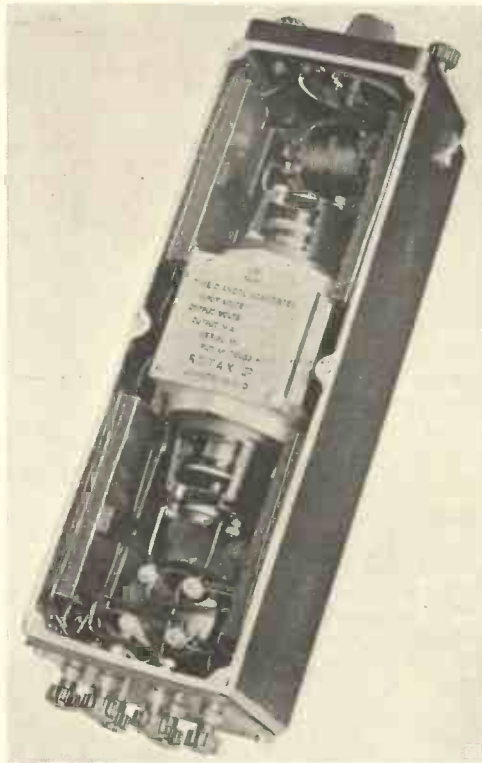
Fig. 1.—AN M-L ANODE CONVERTER WITH LID REMOVED (Rotax Ltd.).
