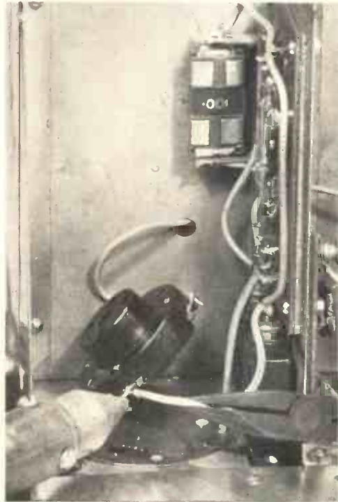
Fig. 30.—METHOD OF REMOVING VALVE HOLDER IN DETECTOR COMPARTMENT.
