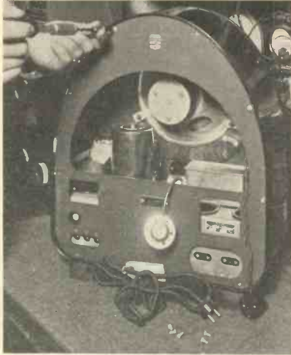
Fig. 2.—FIRST STAGE IN DISMANTLING THE 830A CHASSIS. Removing the back.
