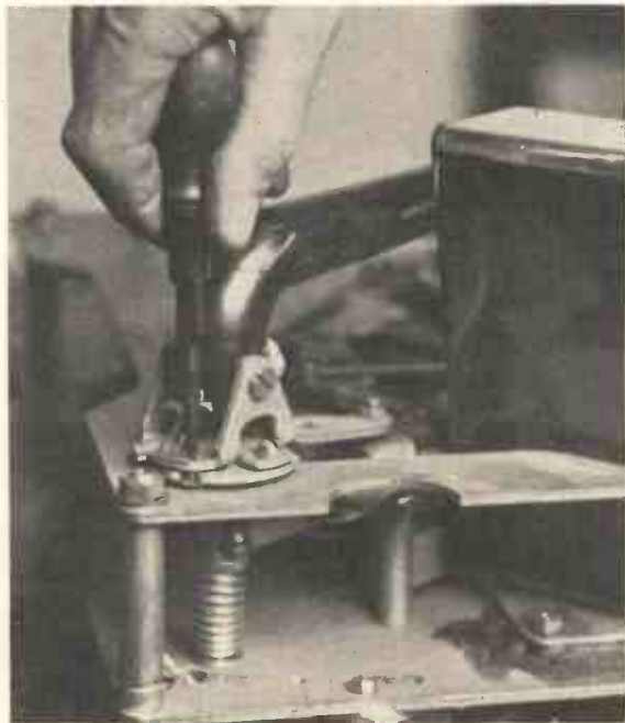
Fig. 7.—ADJUSTING THE DROPPING POSITION OF THE NEEDLE.
