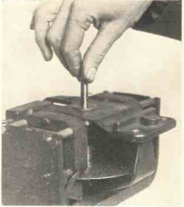
Fig. 5.—THE MOTOR SHOULD BE GENTLY TURNED BY HAND TO DETECT ANY MECHANICAL JAM OR FRICTION.
