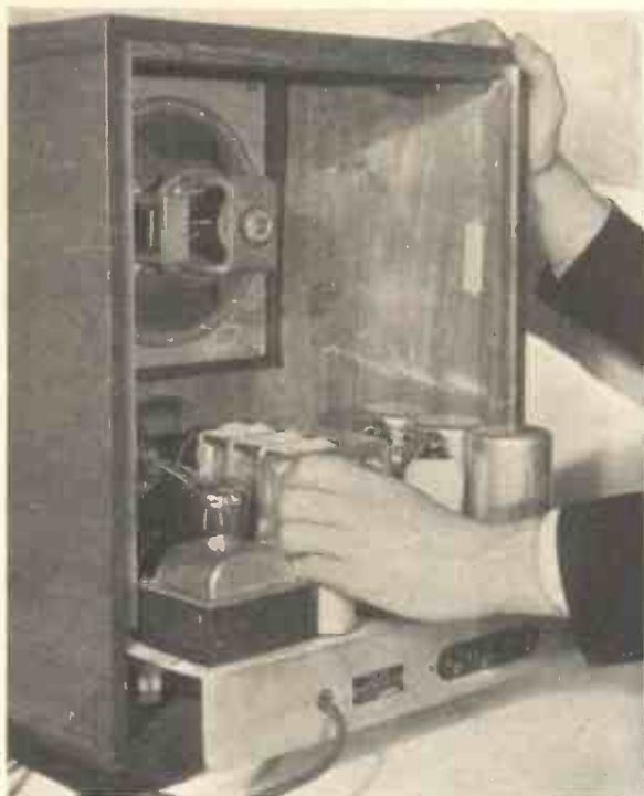
Fig. 3.—DRAW THE CHASSIS STRAIGHT BACK UNTIL THE CONTROL SPINDLES ARE CLEAR OF THE WOODWORK.
