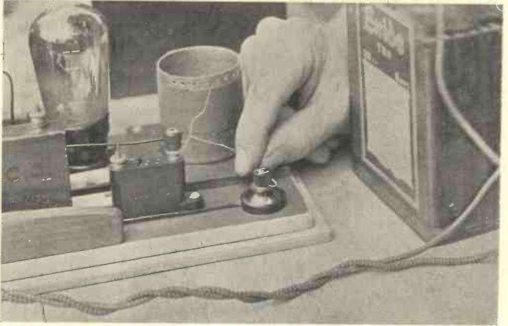
Fig. 13. —CONNECTING BOTTOM LEAD OF COIL TO TERMINAL E.
