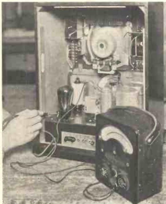
Fig. 7.—CHECKING VOLTAGES AT THE AUXILIARY GRID TERMINAL OF THE PENTODE OUTPUT VALVE.
