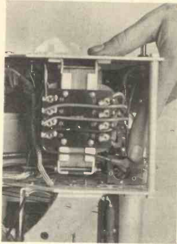
Fig. 4.—THE MAINS AERIAL CONDENSER, C.19.
