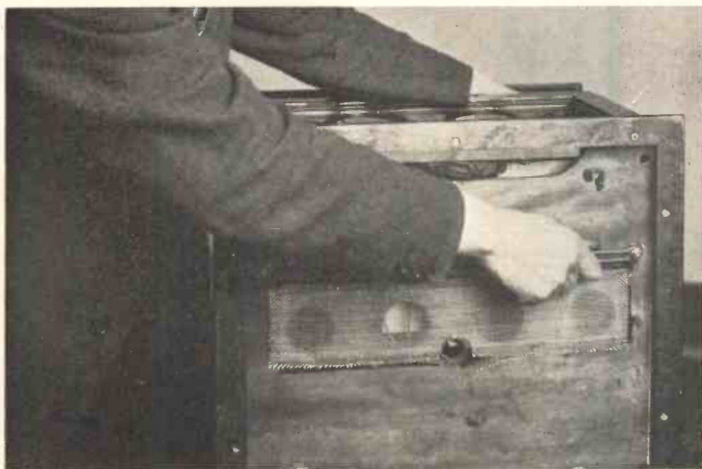
Fig. 10. —REMOVING BOTTOM BOLT WHILE SUPPORTING RADIO UNIT WITH LEFT HAND.
