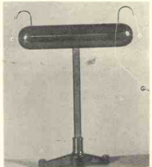
Fig. 27.—A POSITIVE OR NEGATIVE CHARGE CONDUCTED TO A METAL BODY IS DISTRIBUTED EQUALLY OVER THE SURFACE.
