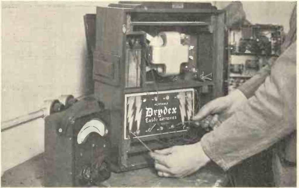
Fig. 23.—TESTING THE HIGH TENSION BATTERY ON LOAD.
