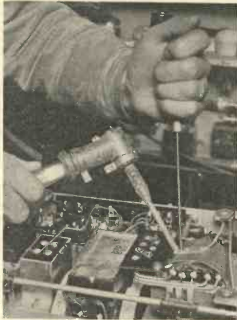
Fig. 25.—REPAIRING THE STRIP TYPE OF FUSE.
