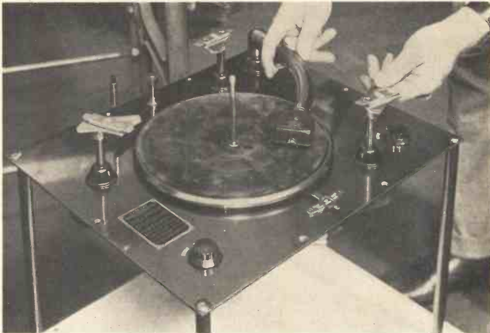
Fig. 30.—HOW THE GARRARD AUTOMATIC RECORD CHANGING UNIT IS ADJUSTED FOR EITHER 10-INCH OR 12-INCH RECORDS.
