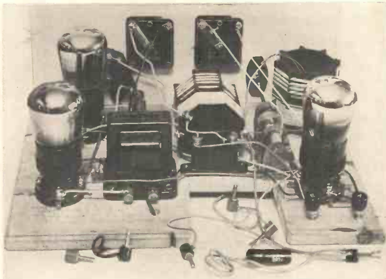
Fig. 9.— THE SET WIRED UP IN READINESS TO PLACE INSIDE CABINET.
