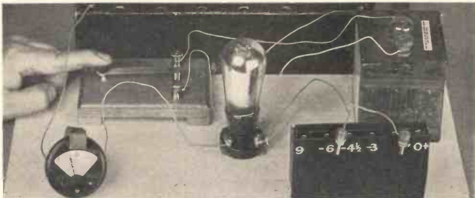
Fig. 22.—HOW THE ANODE CURRENT OF A POWER VALVE IS AFFECTED BY VARYING THE GRID VOLTAGE.
