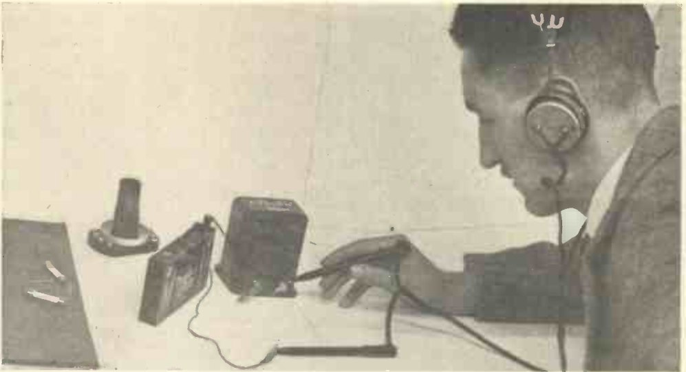
Fig. 6.—METHOD OF TESTING TRANSFORMERS, CHOKES, TUNING COILS, RESISTANCES, ETC. FOR CONTINUITY OF WINDINGS.
