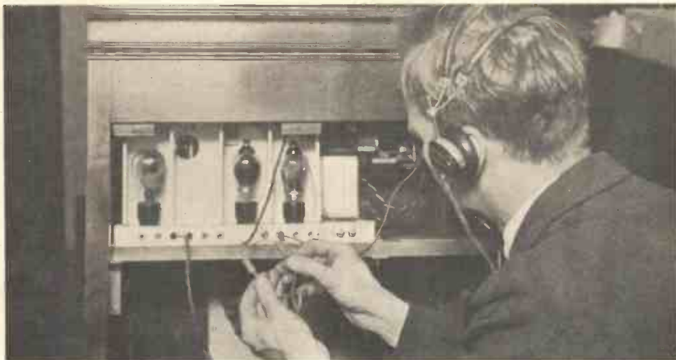
Fig. 12.—TESTING THE OUTPUT OF THE PICK-UP.
