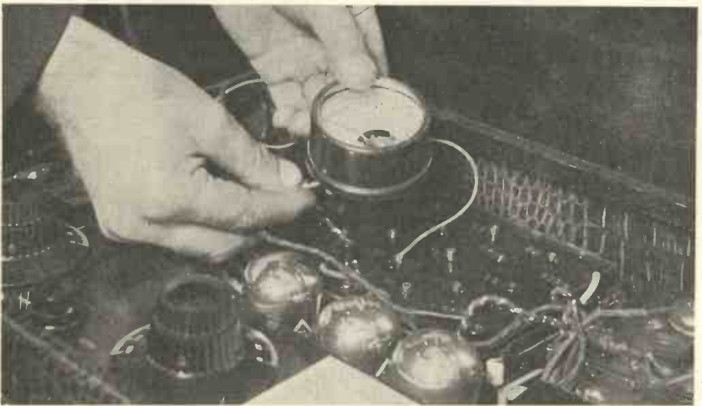
Fig. 3. —TESTING THE CONDITION OF A VALVE WITH A MILLIAMMETER IN THE ANODE CIRCUIT.
