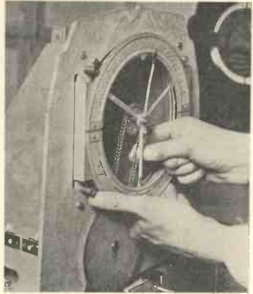
Fig. 12. —METHOD OF ADJUSTING TENSION OF CHAIN DRIVE.
