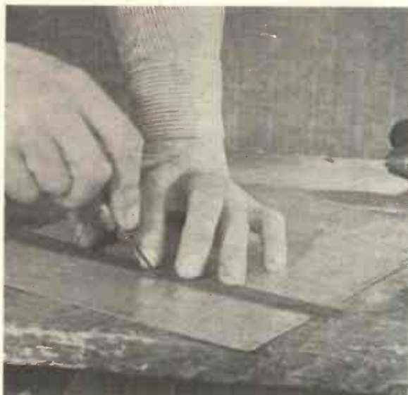
Fig. 3.—USING A SCRIBER TO MARK OUT THE SHEET.
