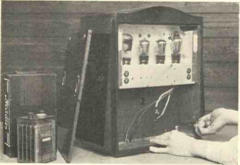
Fig. 10. —HOW TO REMOVE THE CHASSIS OF THE DUPLEX FOUR CABINET ("C") TYPE. FIRST OPERATION.
