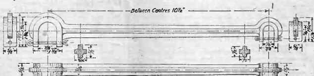
Fig. 6.—Details of the connecting-rod.
