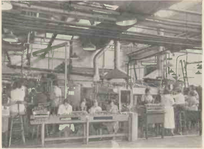
A corner of the Valve Works. In the rear can be seen two of the circular evacuating pumps.
